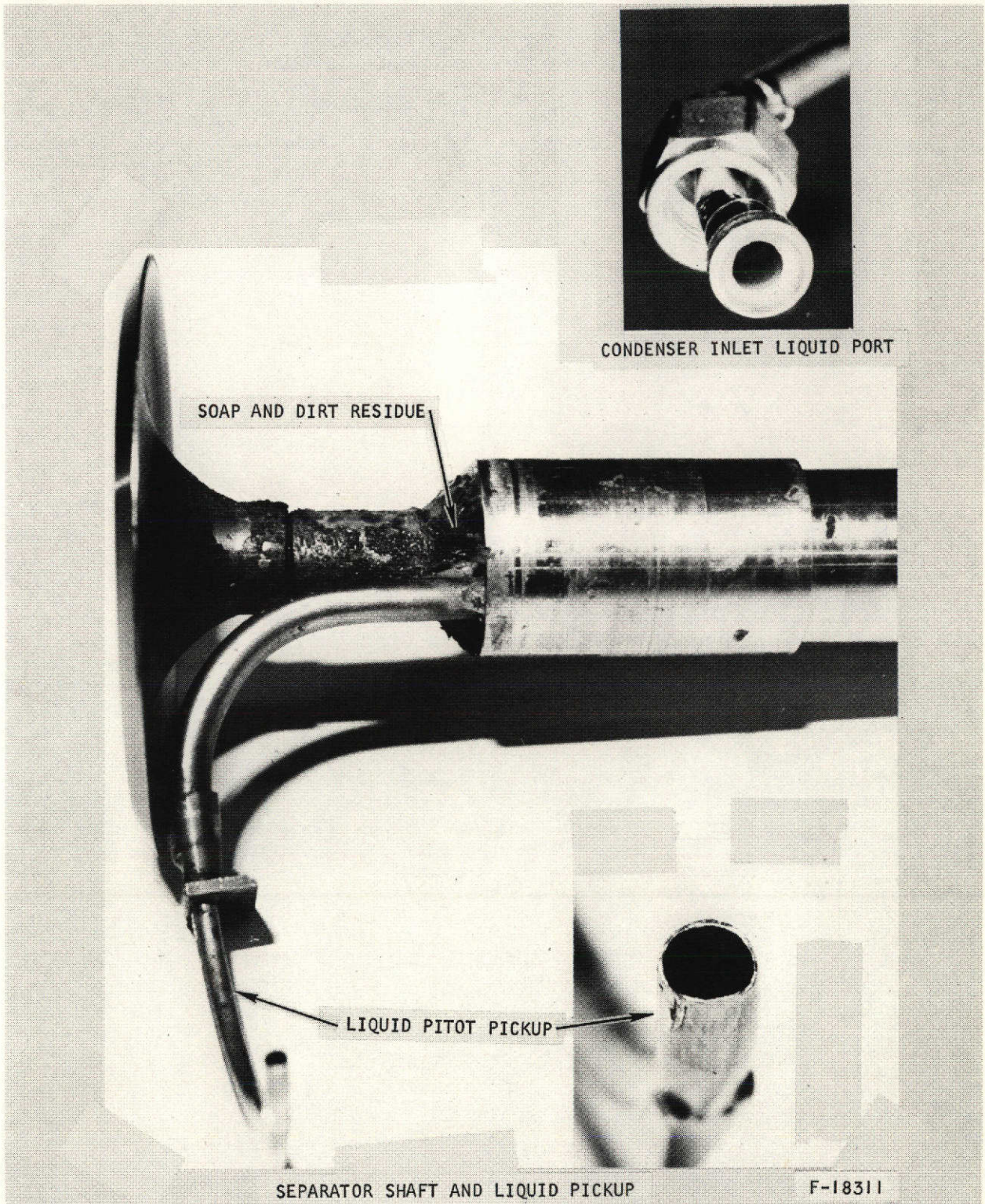
Figure 3-16. Post Phase I Examination, Appearance of Separator Shaft Assembly and Condenser Liquid Inlet Port
