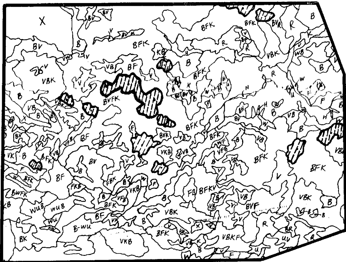
Figure 1.4. Skylab interpretation of principal resource types in the crest region of the Feather River watershed. The 300 mi 2 area above is mapped at a scale of 1:250,000 and required 2 hours interpretation.
