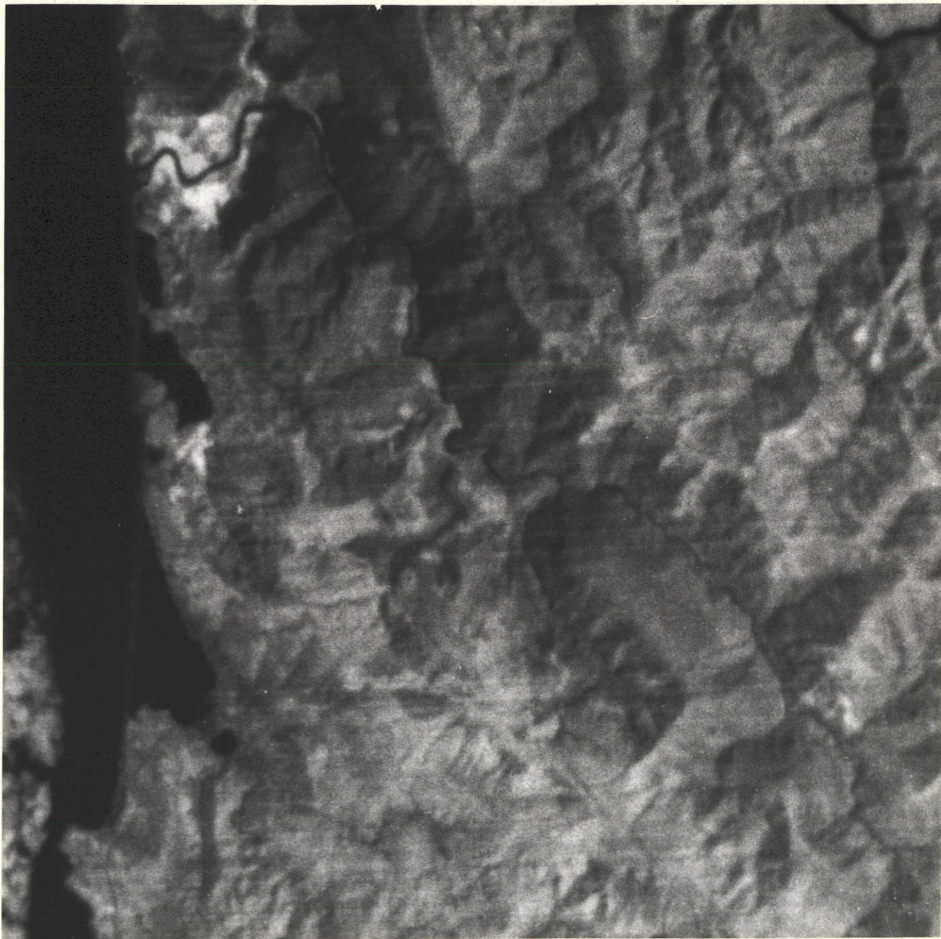
Figure 4.31. This 1:125,000 scale image was obtained from an ERTS-1 April 6, 1973 Band 7 (1:1,000,000) transparency. It is apparent that information on landform characteristics and the extent of bays, lagoons, and large stream channels is readily extractable from Band 7 imagery. However, Band 7 is generally not useful, in the region examined, as an information source for land use, vegetation type, period since forest harvest, or sediment plume detection. In the above figure note the general absence of harvest boundaries (except in the case of the twelve to seventeen year post-harvest areas and in some instances old growth forest adjacent to harvested areas), vegetation boundaries, and the sediment plume known to be present on the same date from Figure 4.30.
