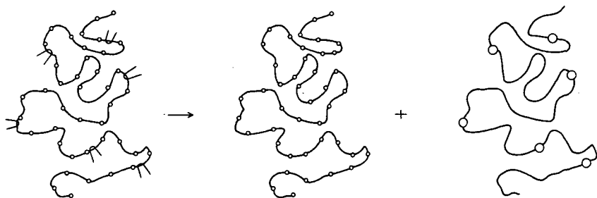
FIGURE 7.—In the Chomppf-Duiser-Prins entanglement theory an (m-1) -entangled bead-spring molecule having (N+1) beads is treated as the sum of an unentangled molecule having (N+1) beads and an unentangled molecule having (m-1) high-friction beads.
