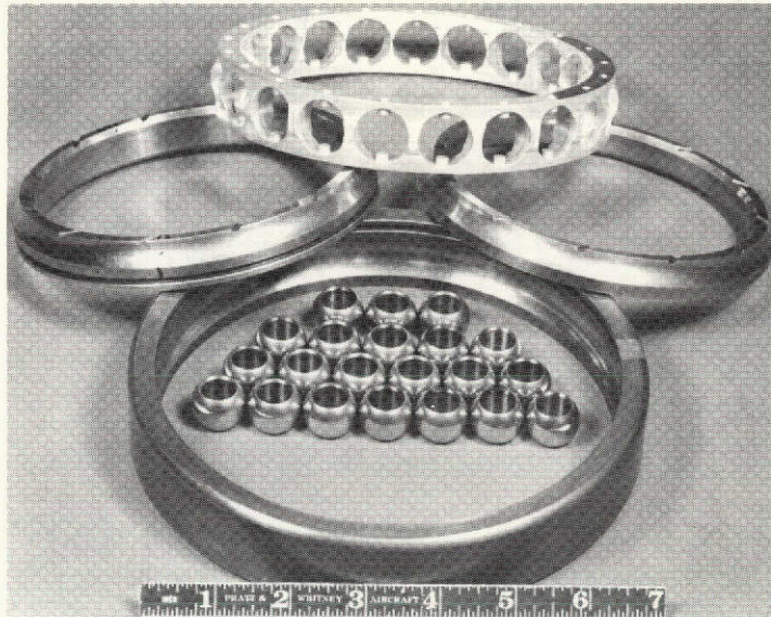
Figure 1. - Drilled-ball bearing with 125-millimeter-diameter bore tested in reference 8 and used for analysis in present report.
