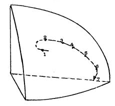
Waypoints 2 through 6 define the en route RNAV path. The system switches to new waypoint-centered reference frames as the flight progresses. The spacing between waypoints must be less than 500 km for good free inertial performance. The system will insert waypoints as necessary to keep the coordinate centers within the limits. Waypoint #7 is the coordinate center at the landing runway.
