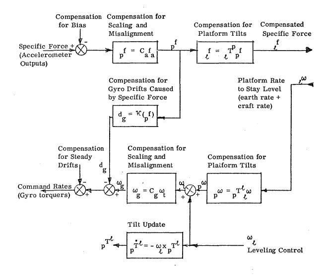
Figure 5. - Block Diagram of Software Compensation for IMU Anomalies
