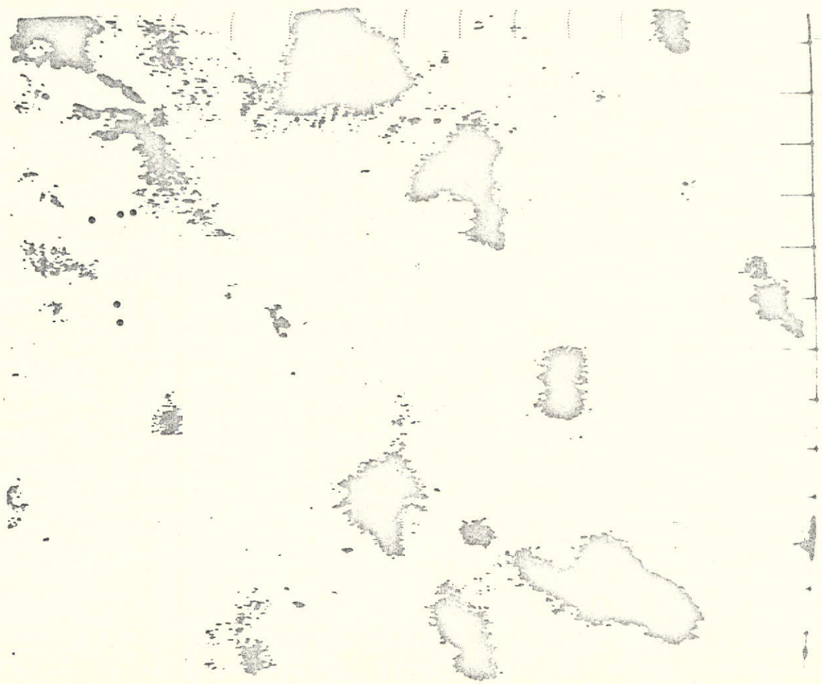
Figure 6c.--Thematic mask of Tucson Test Site showing areas where MSS-6/MSS-5 \geq 1.25/1.00 . Location of five ground-truth stations shown in upper left (solid circles). December 26, 1972.
