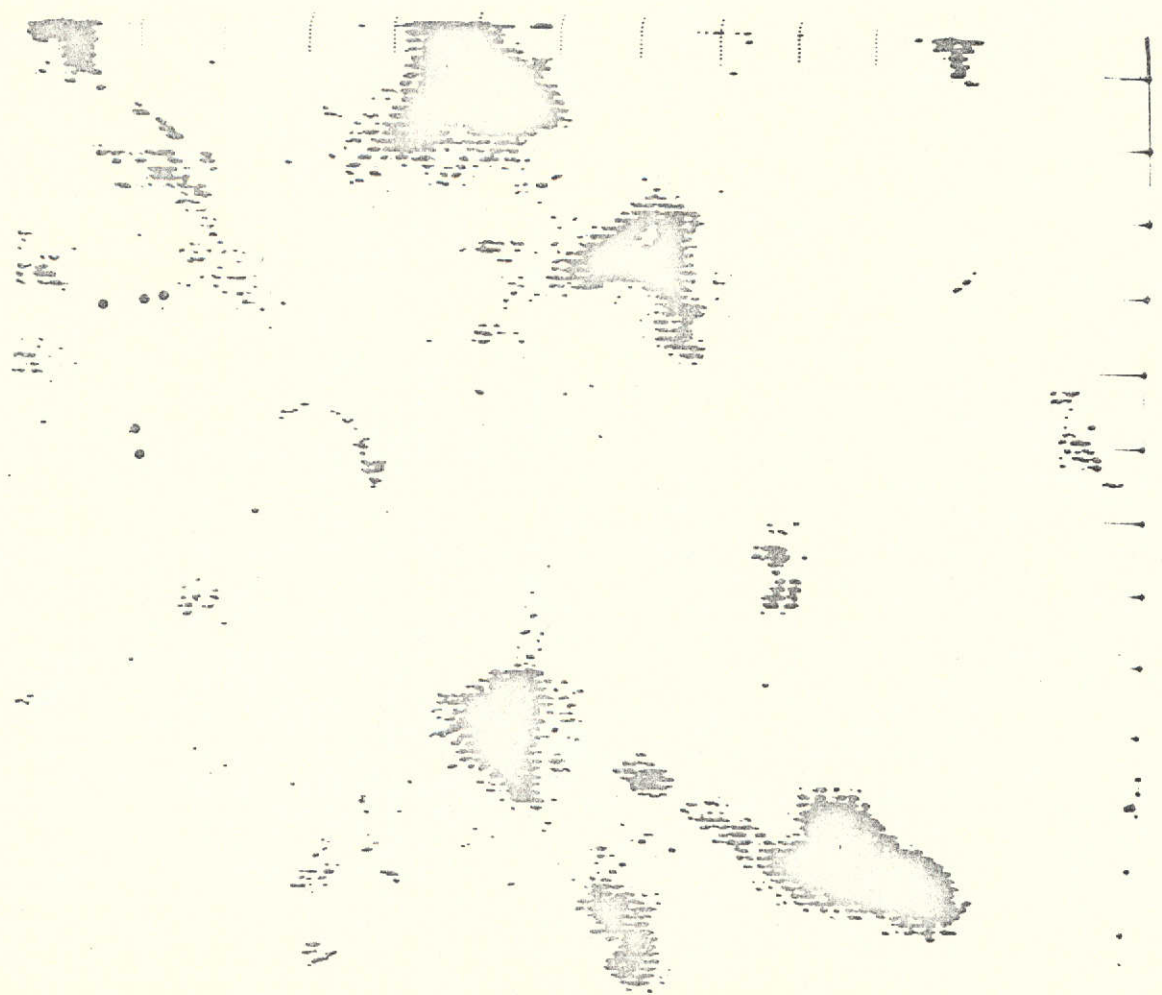
Figure 6d.--Thematic mask of Tucson Test Site showing areas where MSS-6/MSS-5 = 1.25/1.00 . Location of five ground-truth stations shown in upper left (solid circles). January 13, 1973.
