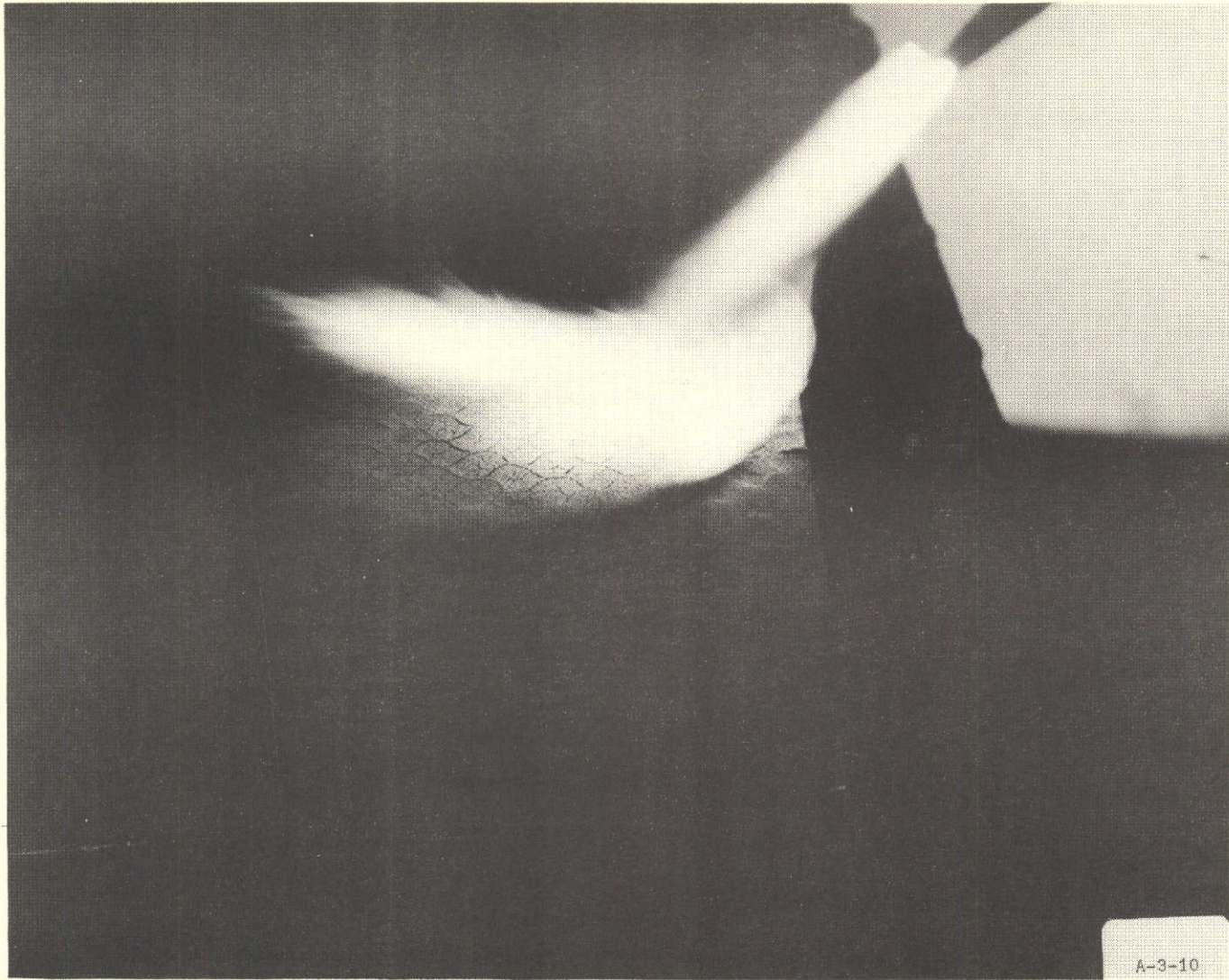
Figure 6 Flame Test of Ablative Panel
