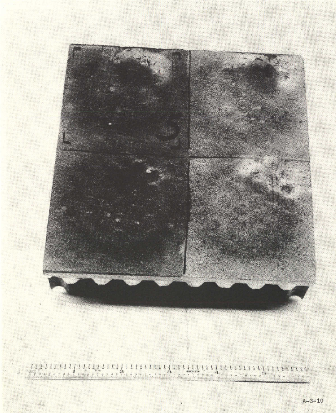
Figure 7 Ablative Test Panel After Flame Test
