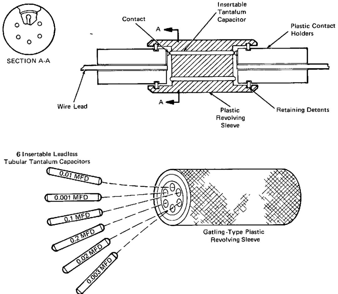
Due to circuit deterioration, component tolerance changes, and changes caused by extreme environmental conditions, adjustments have to be made in the capacitance of RC networks of certain electrical/electronic circuits. The present methods of changing capacitance include a patch cord plug-in unit that allows switching from one capacitor in the patch cord unit to another.
