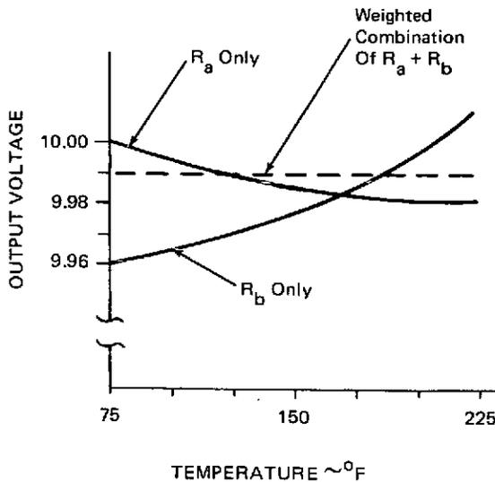
Figure 2. Typical Output Temperature Coefficients
