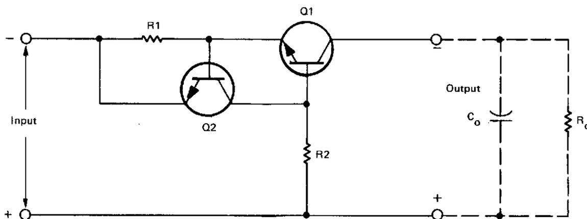
The primary purpose of this circuit (see fig.) is to limit current surges during power turn-on of DC sources. The circuit has application in systems where current limiting is required during power sequencing.
