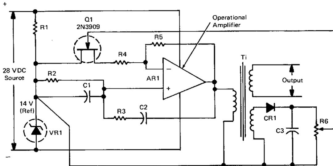
This circuit (see figure) illustrates the use of an additional secondary winding on a transformer to provide an isolated feedback circuit for load regulation. The feedback source is connected after the output stage, yet it provides for isolation between load and feedback circuit. Usually, feedback circuits are connected to the load or connected ahead of the output stage.
