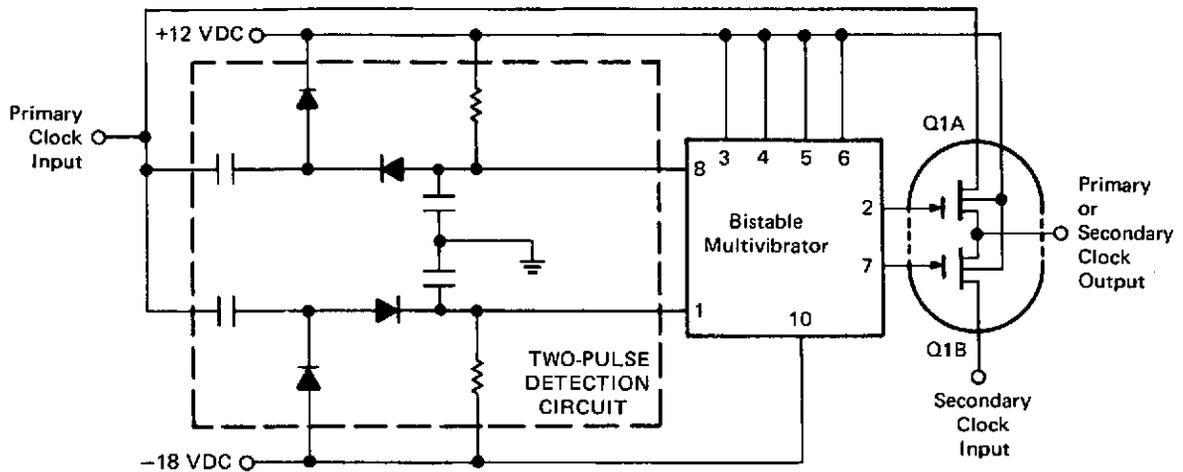
The circuit shown in the figure is designed to switch from a primary clock input to a secondary clock input if the primary clock input is not received for four or more counts.
