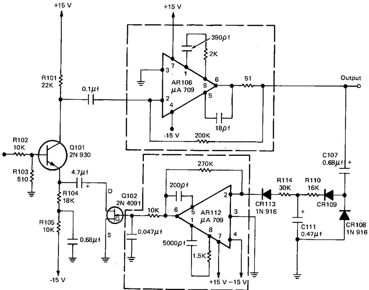
circuit resistance occurs when the field effect transistor (FET) Q102 changes its resistance to ground. When the FET is open, the emitter of transistor Q101 sees only the 18K resistance R104, and the stage gain is minimum. When the FET is closed, i.e., the source to drain resistance of the FET reduces to about 30 to 40 ohms under control of a signal at the gate, the 30 to 40 ohms resistance is in shunt with the 18K resistance of R104, providing maximum gain for the Q101 amplifier stage.
