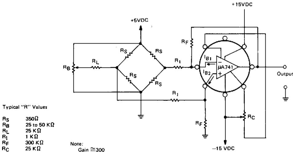
Many integrated circuit operational amplifiers provide taps for external balance circuits to facilitate output offset adjustment. In the typical application (see figure), offset is provided by the  $R_B$  and  $R_1$  network which is normally associated with a bridge type transducer ( $R_S$ ). In this application, the amplifier offset taps are available for temperature compensation.
