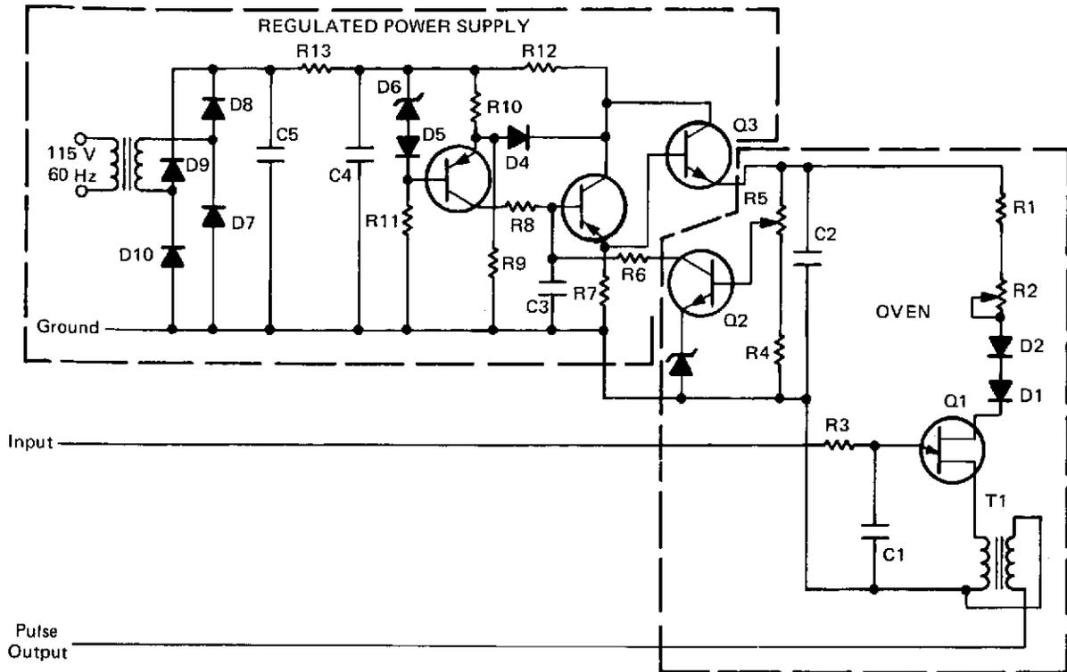
The circuit shown in the figure is a precise fixed reference voltage variation detector. The tolerance detector consists of a unijunction transistor relaxation oscillator trigger circuit and stable power supply with the trigger circuit components and the voltage reference components of the power supply mounted in a single oven for common temperature environment.
