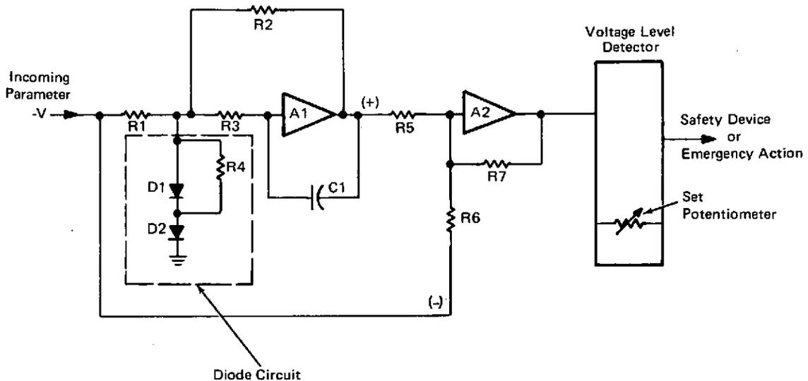
A circuit has been designed to obtain a voltage signal that will initiate timely action in case the rate-of-change of a selected, measured parameter (temperature, pressure, flow, etc.) exceeds a pre-determined limit.
