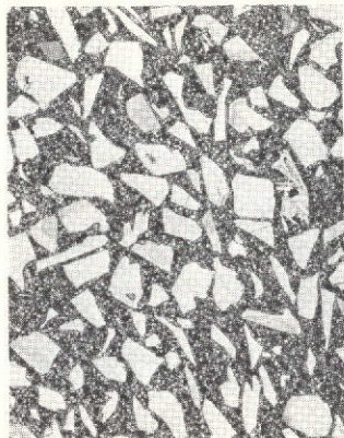
NORTON LOW FIRED SiC DUPLIX GRAIN SIZE: 100 \mu\text{m} , 4 \mu\text{m}
