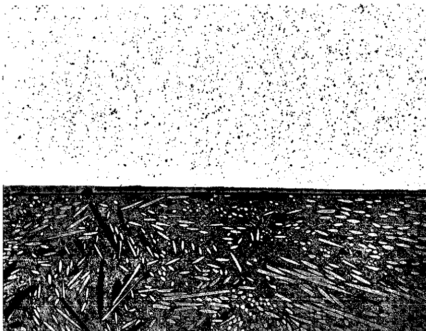
Figure 18. Sample R-3 Showing Reaction Sintered \text{Si}_3\text{N}_4 and Cap of Inconel 702 After Attempted Infiltration.
