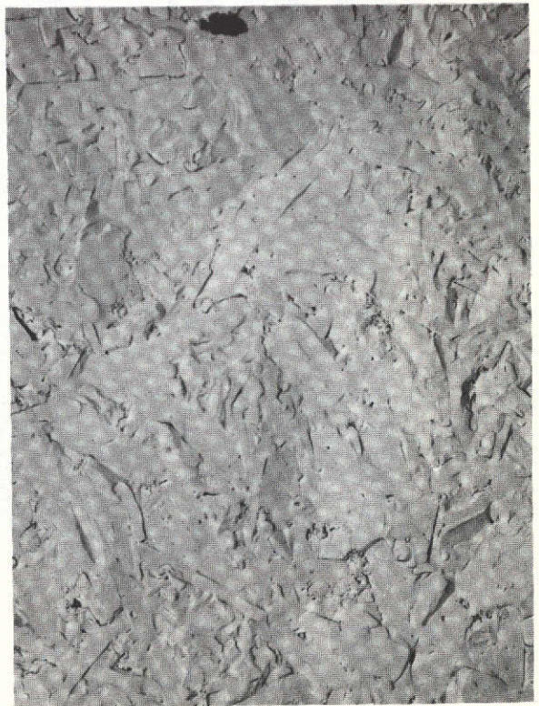
Figure 12. Microstructure of SiC Billet D1823 Pressed at 2140°C - 4000 psi - 40 min. using PPG Industries' Powder (a) As-polished, (b) Etched, and (c) Replica of Fracture Surface.
