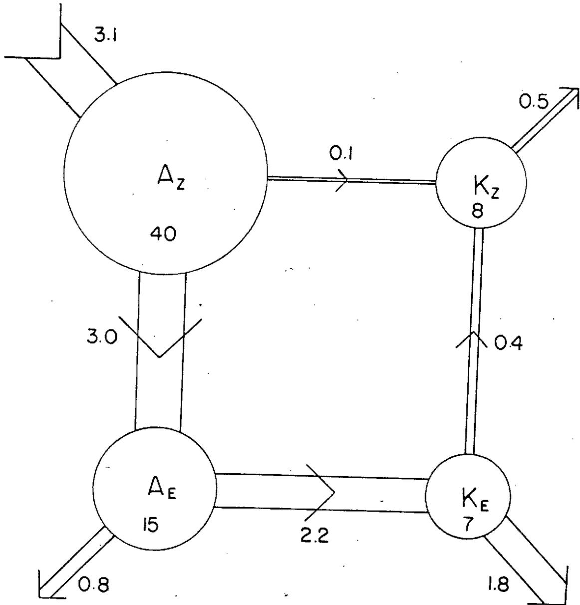
Fig. 1. The energy cycle of the atmosphere as estimated by Oort (1964). Values of energy are in units of  $10^5$  joules  $m^{-2}$ , and values of generation, conversion and dissipation are in watts  $m^{-2}$ .
