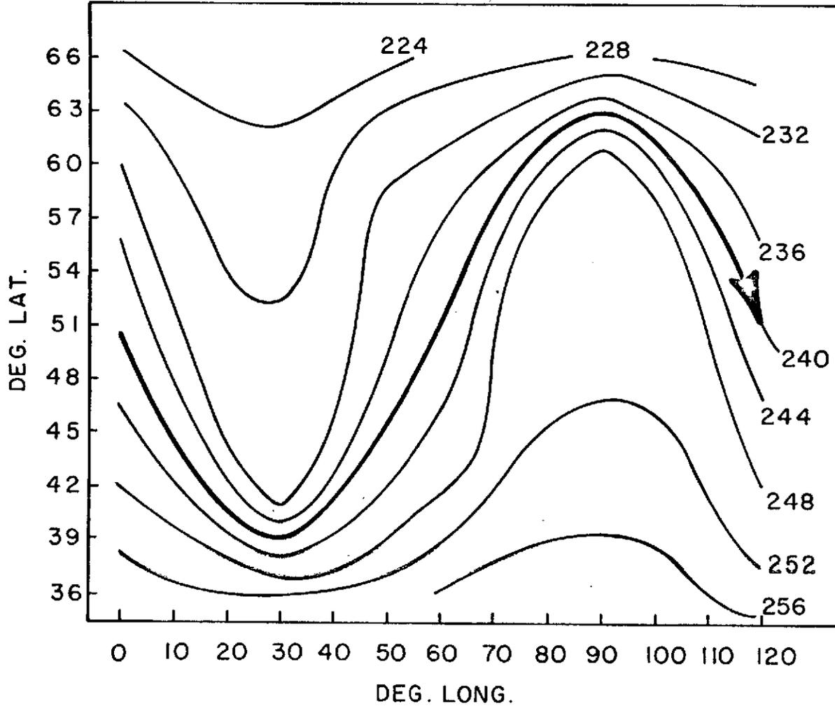
Fig. 2. Schematic illustration of jet-stream level flow and the distribution of underlying layer-mean temperature. The jet axis, the heavy line with arrow-head, is a line joining the maximum wind speeds. The surface wind speed is assumed to be zero everywhere. Hence jet-stream level streamlines are parallel to the layer-mean isotherms ( $^{\circ}\text{K}$ ).
