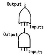
The OR GATE describes the logical operation whereby the output is caused by the occurrence of any of the inputs.
