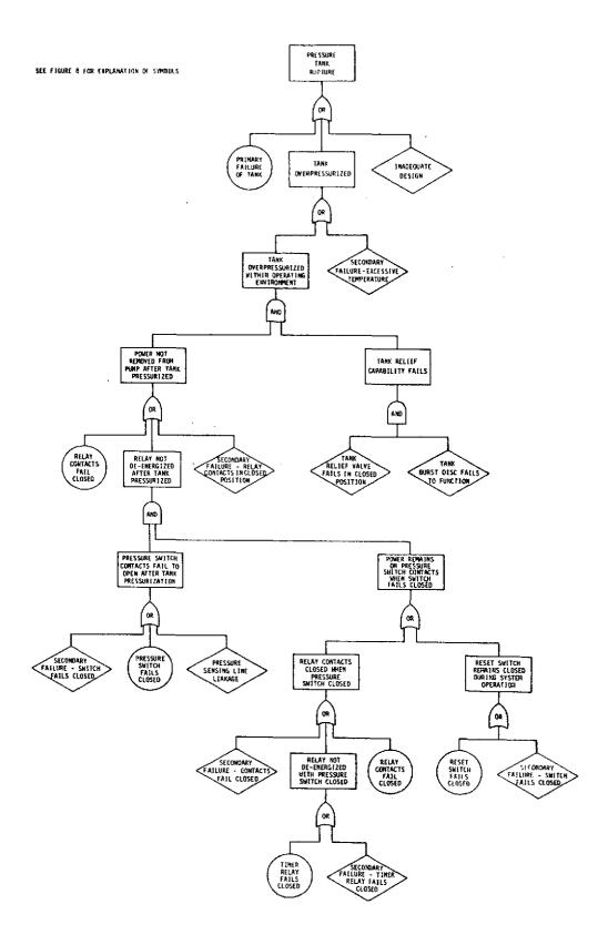
FIGURE 7. LOGIC FOR PRESSURE TANK RUPTURE
