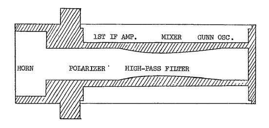
Figure 3-5 Cross-sectional View of Waveguide-MIC System (2) (alternative [C])
