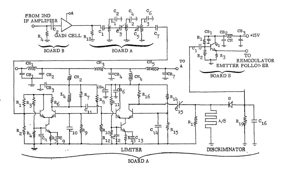
Figure C-8 Circuit Diagram of the Limiter and Discriminator of the Indoor Unit
