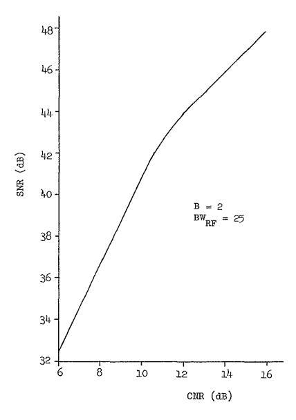
Figure 5-10 Measured SNR vs CNR
