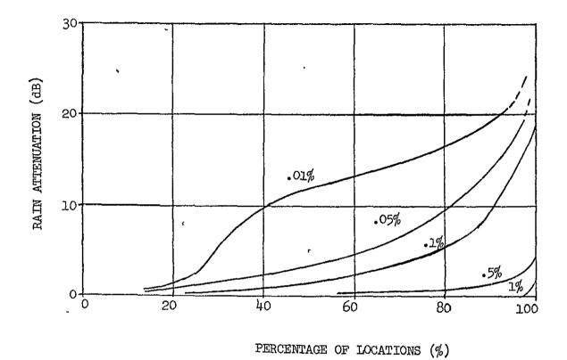
Figure 5-8 Rain Attenuation vs. Percentage of Locations in the U.S.A. for the 12 GHz Signals Broadcast from Satellites (Studied by COMSAT [6]. Parameter is percentage of outage)
