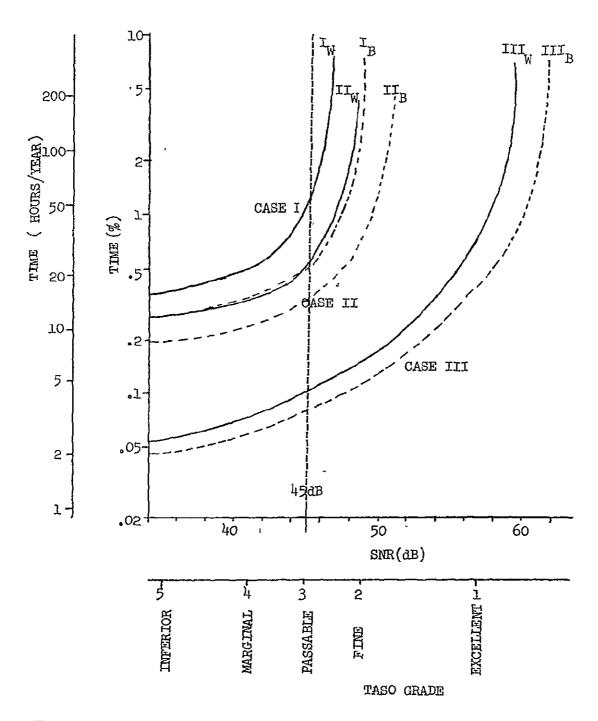
The solid lines show the best cases where probabilistic degradation except rain attenuation is not encountered (noted by B). The dotted lines show the worst case, on the other hand (noted by W). For outage; 12 hours a day of service is assumed. (12 GHz).
