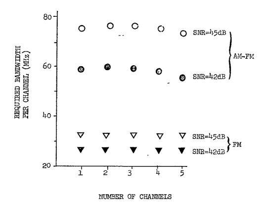
Figure D-5 Required Bandwidth per Channel vs the Number of Channels
