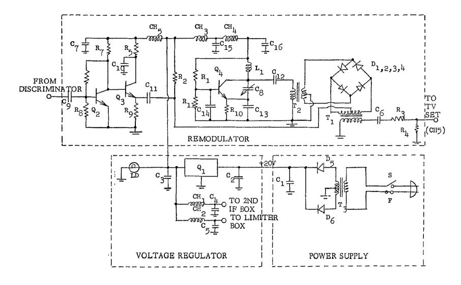
Figure C-9 Circuit Diagram of the Remodulator, Voltage Regulator and Power Supply of the Indoor Unit
