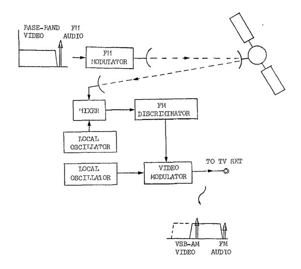
Figure 2-3 Block Diagram of the FM System
