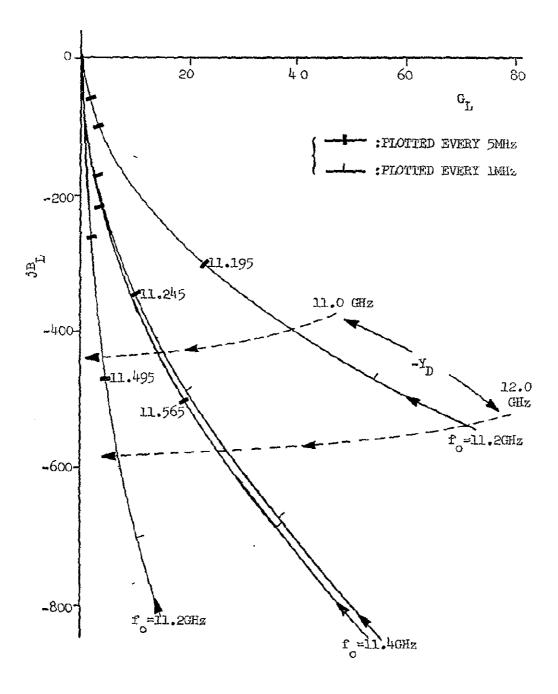
Figure A-4 Normalized Admittance ( $Q_0 = 20,000$ ; K = 25;  $f_m = 11.4$  GHz;  $f_0 = 11.2$  and 11.4 GHz)
