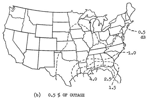
Figure 5-5 Rain Margin Map for the 12 GHz Signal for 0.1 and 0.5% of Outage (studied by COMSAT[6])
