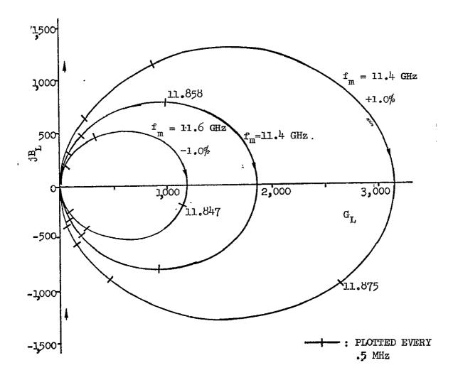
Figure A-9 Effect of  $f_m$  on  $Y_L$  ( $Q_o = 20,000$ ; K = 25;  $f_o = 11.8$  GHz;  $f_m = 11.4$  GHz and 11.4 GHz + 1%).
