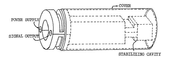
Figure 3-4 Sketch of Assembled Packaging (alternative [B])
