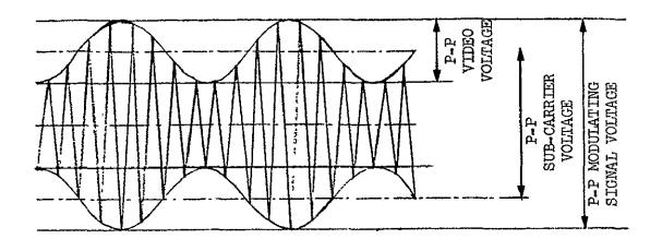
Figure 2-6 Waveform of the VSB-AM Video Signal (modulating signal of the AM-FM system)
