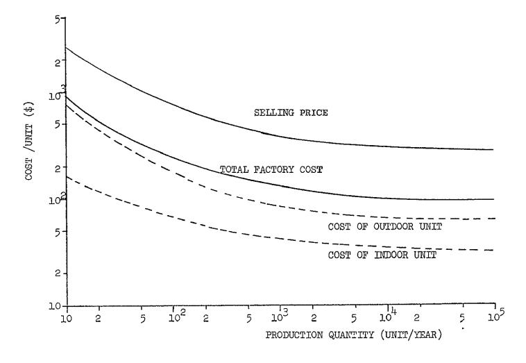
(Total factory cost is the sum of an outdoor unit cost and an indoor unit cost; selling price is the total factory cost multiplied by 3.0)
