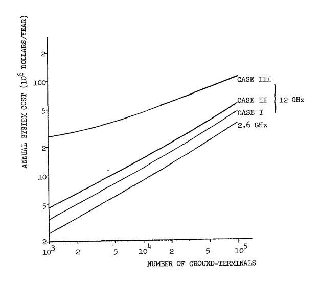
Figure 5-9 Annual System Cost vs Number of Optimum Ground-Terminals for the 2.6 GHz and the 12 GHz Systems
