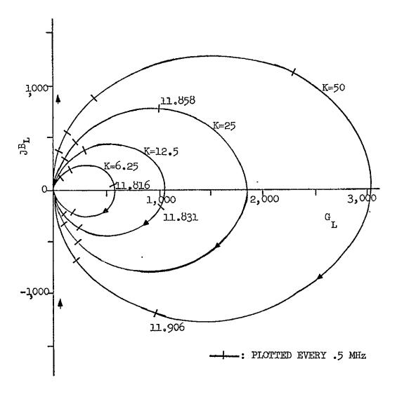
Figure A-8 Effect of K on Y<sub>L</sub> ( $Q_o = 20,000$ ;  $f_m = 11.4$  GHz;  $f_o = 11.8$  GHz; K = 50, 25, 12.5 and 6.25).
