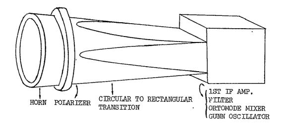
Figure 3-2 Sketch of Waveguide System (alternative [A])
