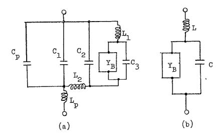
Figure A-5 Equivalent Circuit of Gunn Diode
