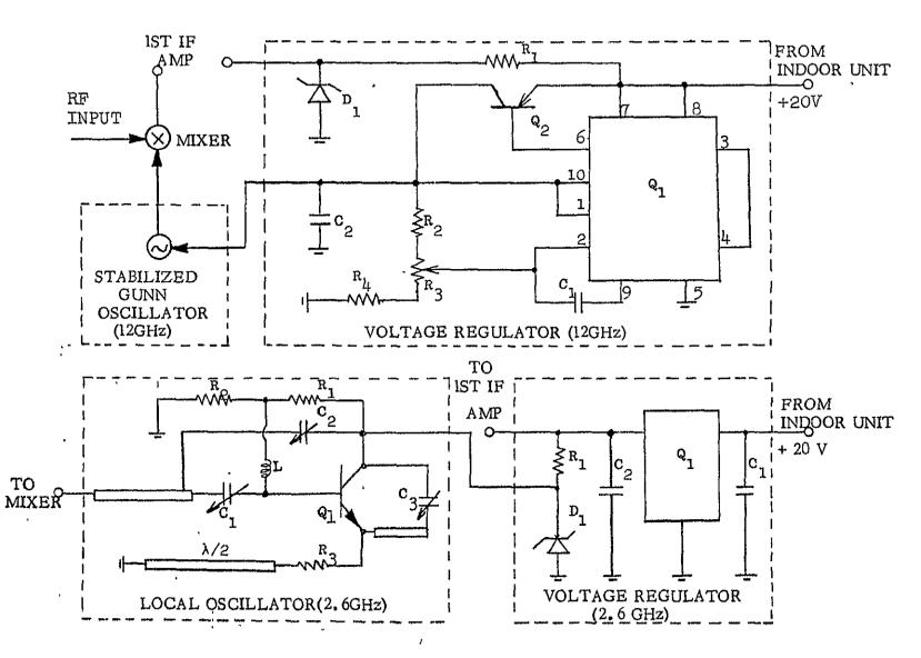
Figure C-5 Circuit Diagram of the Front-end and the Voltage Regulator of the Outdoor Unit
