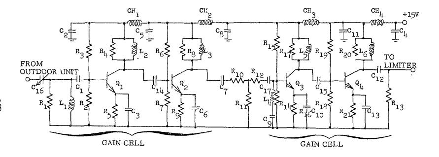
Figure C-7 Circuit Diagram of the Second IF Amplifier Circuit of the Indoor Unit
