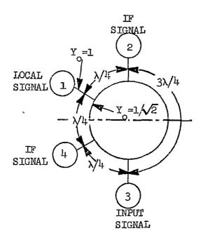
Figure C-2 Principle of Rat-Race Hybrid Mixer
