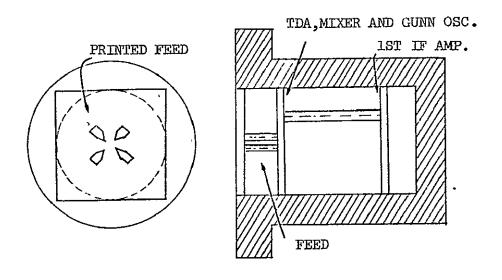
Figure 3-6 Sketch of MIC System (alternative [D])
