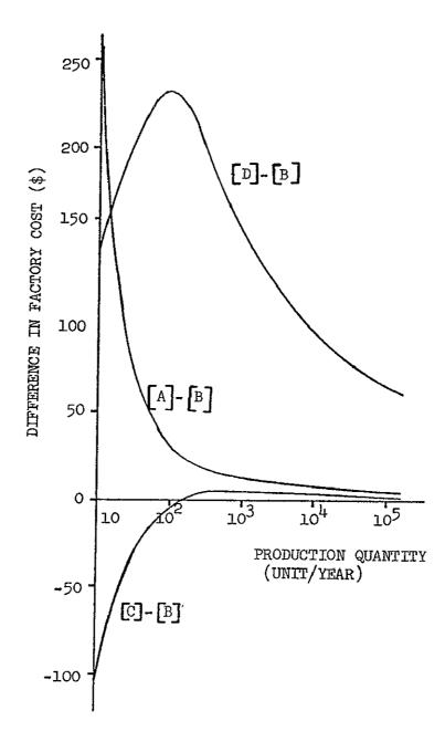
Figure 3-7 The Difference in Cost of Alternative [A], [C] and [D] from Alternative [B]
