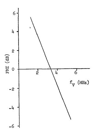
(BW  $_{rf}$  = 25.0 MHz and FMI for FM systems with the same bandwidth = 15.5 dB)
