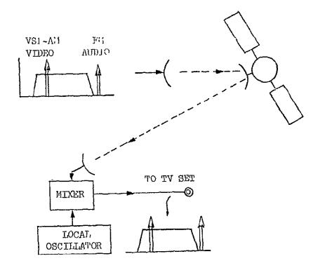
Figure 2-4 Block Diagram of the AM System
