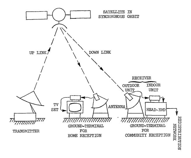
Figure 1-1 Block Diagram of Direct Reception from Broadcasting Satellite
