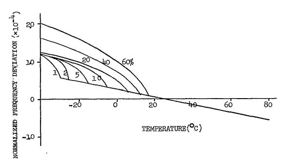
Figure A-11 Normalized Frequency Deviation of Sealed Invar Cavity (Parameters are initial humidity. Thermal expansion rate =  $1.0 \times 10^{-6}$ /°C. Actual temperature region to be considered is between -15°C and 80°C.)
