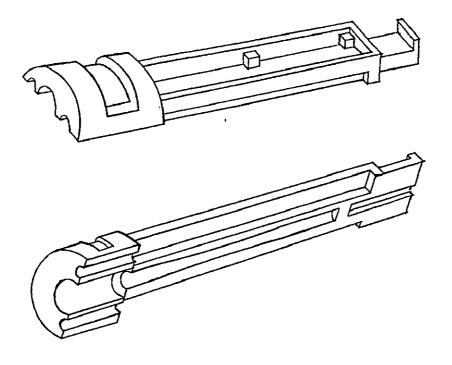
Figure 3-3 Sketch of Cast Packaging (alternative [B])
