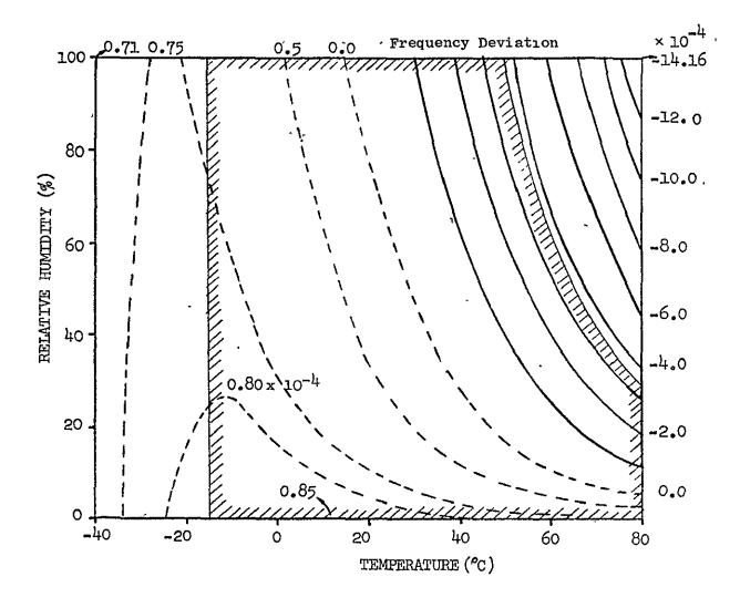
Figure A-10 Normalized Frequency Deviation Contours of the Invar Cavity (Thermal expansion rate =  $1.0 \times 10^{-6}$ /°C and air pressure = 700 mmHG. Broad lines show actual region to be considered)
