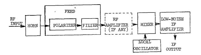
Figure 3-1 Block Diagram of Outdoor Unit
