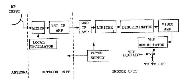
Figure B-3 Block Diagram of the Ground-Terminal
