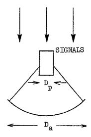
Figure C-4 Blockage of Signals by Packaging
