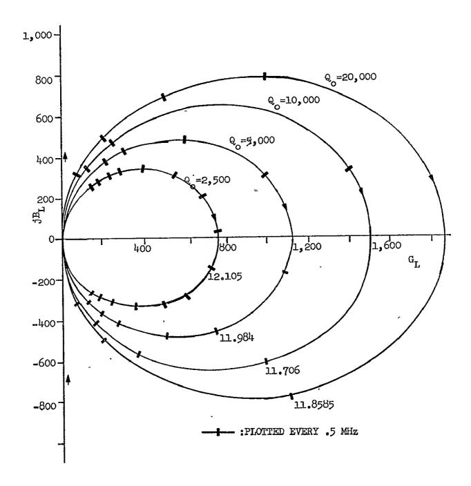
Figure A-7 Effect of Q on Y<sub>L</sub> (K = 25;  $f_m = 11.4$  GHz;  $f_o = 11.8$  GHz;  $Q_o = 20,000, 10,000, 5,000$  and 2,500).
