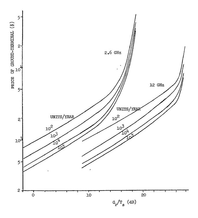
Figure 5-4 Optimized Ground-Terminal Selling Price vs  $G_r/T_s$  at Various Production Quantities for the 2.6 and the 12 GHz Systems
