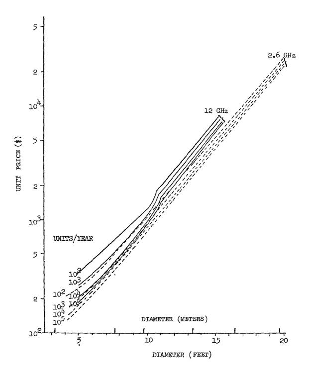
Figure 5-2 Installed Antenna Price vs Diameter for 2.6 and 12 GHz Systems
