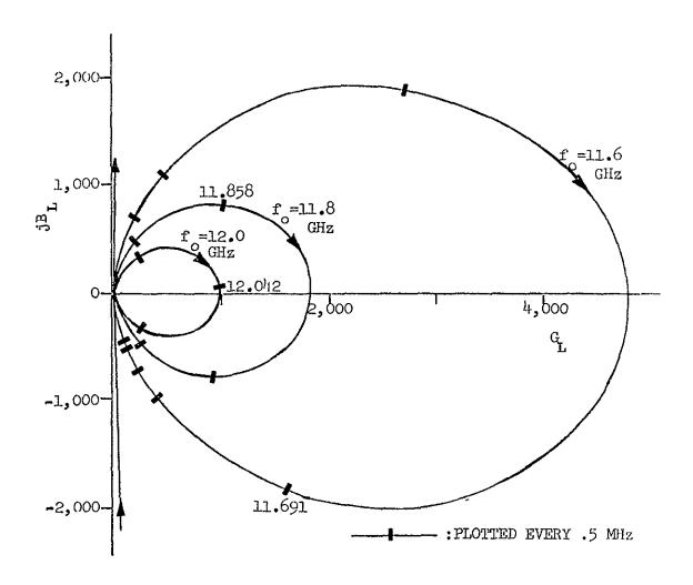
Figure A-3 (a) Normalized Admittance Y - effect of f (
