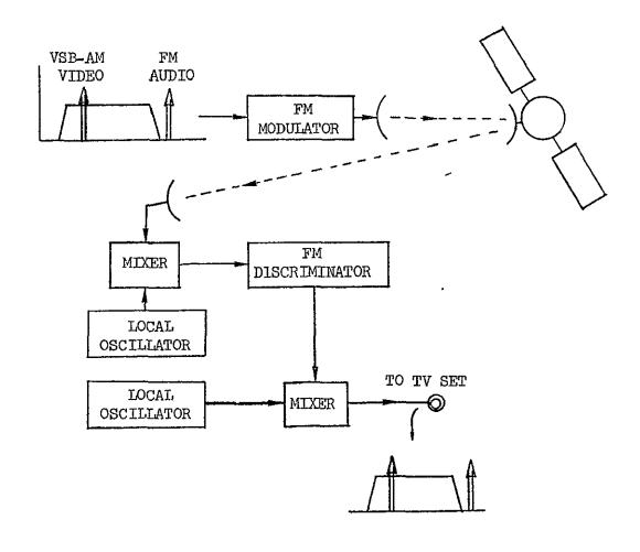
Figure 2-5 Block Diagram of the AM-FM System
