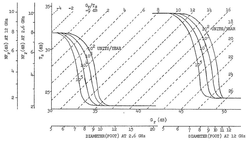
Figure 5-3 Optimum Ground-Terminal (combination of antenna and receiver) for the 2.6 and the 12 GHz Systems at Various Production Quantities Per Year and G /T (55% antenna efficiency and 50°K (100°K) of antenna temperature for the 2.61 (12) GHz are assumed)
