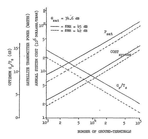
Figure 5-7 Annual System Cost, Satellite Transmitter Power and Ground-Terminal  $G_r/T_s$  at the Optimum for Various Numbers of Ground-Terminals for the 2.6 GHz System
