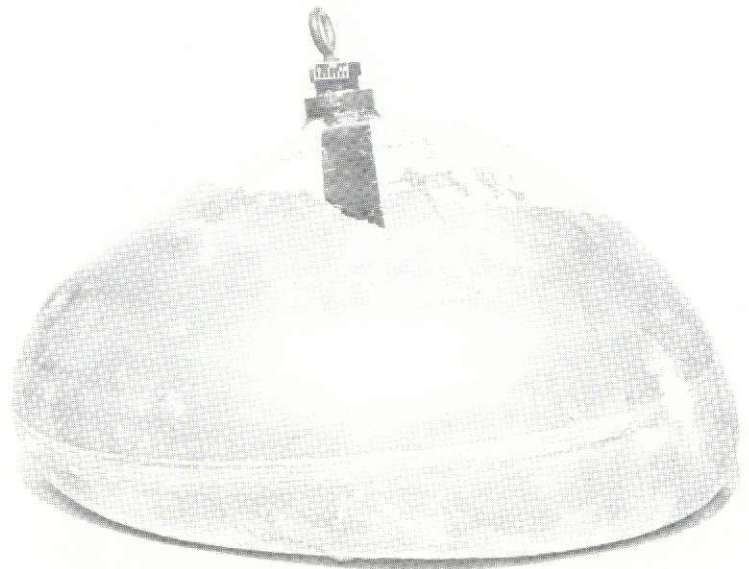
Figure 12(b), - Nuclear containment system - after impact at 1055 ft/sec.
