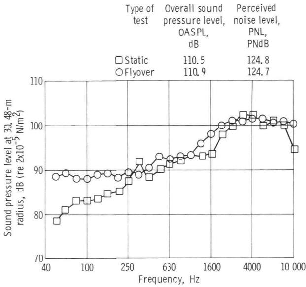
Figure 12. - Comparison of flyover and static spectra for 48-tube suppressor nozzle. Relative jet velocity,  $V_r$ , 504 m/sec (1654 ft/sec); angle of peak noise flyover (acoustic angle),  $\theta$ ,  $70^\circ$ ; 1/3-octave bands.
