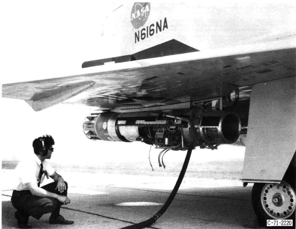
Figure 3. - Nacelle modification for static tests.
