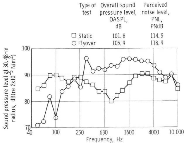
Figure 14. - Comparison of flyover and static spectra for 48-tube suppressor nozzle with scoops plus acoustic shroud and plug. Relative jet velocity,  $V_r$ , 501 m/sec (1642 ft/sec); angle of peak noise for flyover (acoustic angle),  $\theta$ ,  $30^\circ$ ; 1/3-octave bands.
