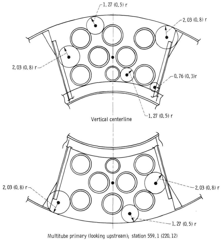
Figure 7. - Primary base static pressure instrumentation. Dimensions are in centimeters (in.).
