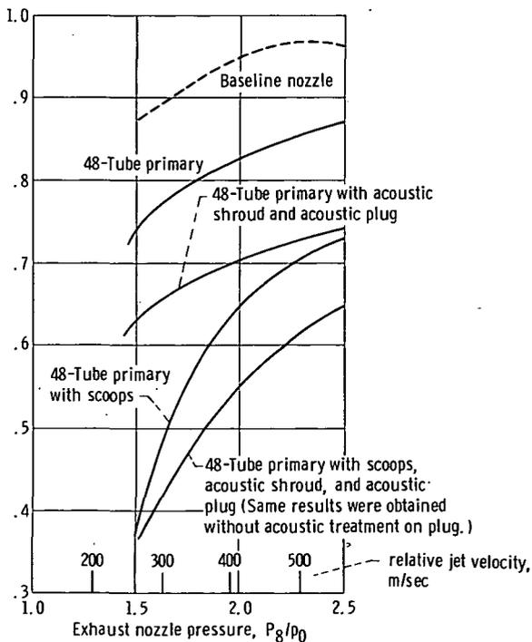
(b) Flyover tests. Flight Mach number,  $M_0$ , 0.4; corrected secondary weight flow ratio,  $\omega\sqrt{T}$ , 0.06.
