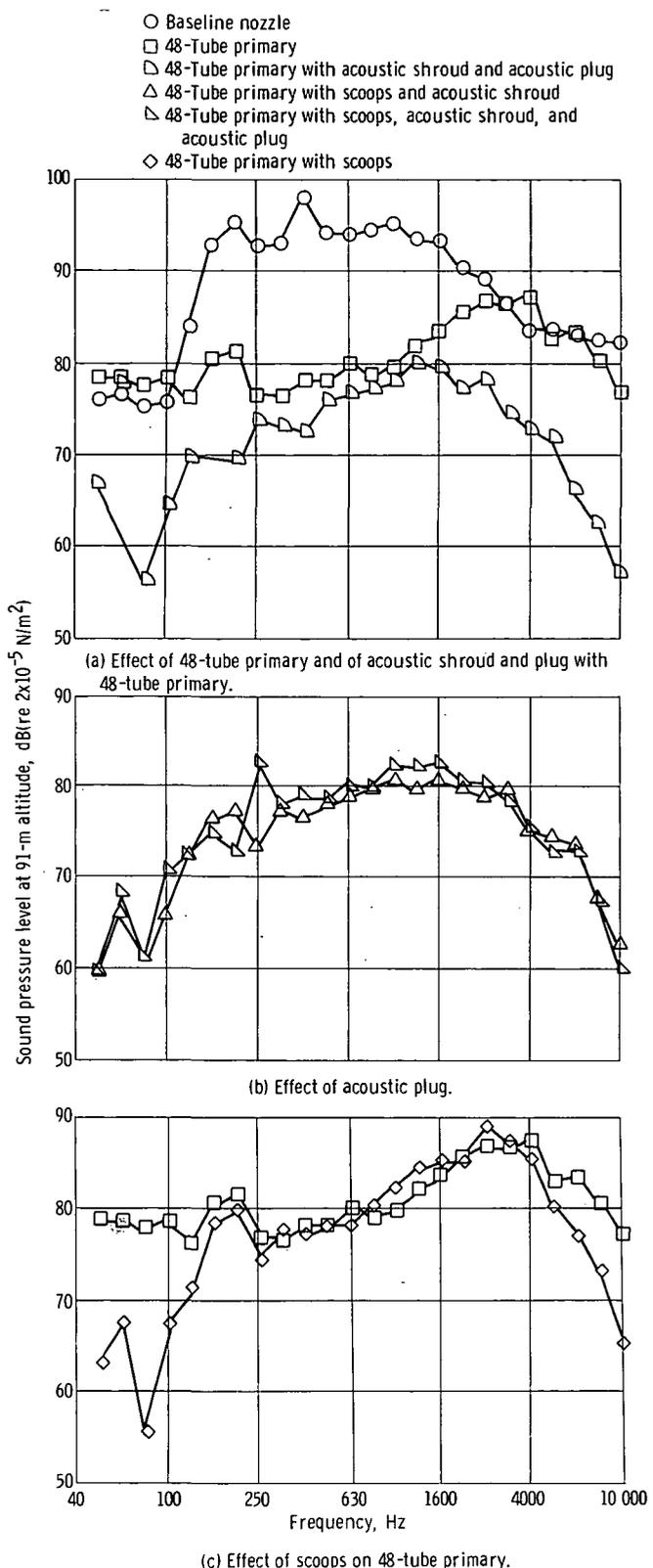
Figure 18. - Comparison of flyover spectra. Relative jet velocity,  $V_r$ , 502 m/sec (1646 ft/sec); acoustic angle (angle of peak noise for plug at flyover),  $\theta$ ,  $40^\circ$ ; 1/3-octave bands.
