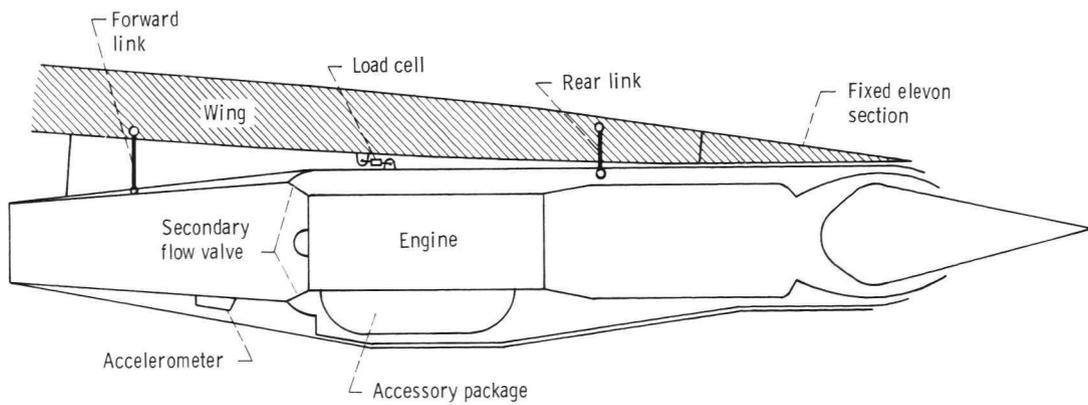
Figure 2. - Nacelle-engine installation.
