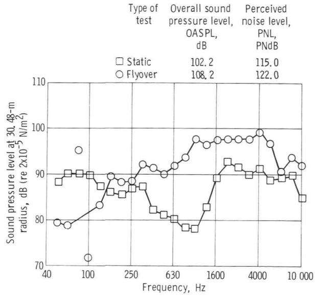
Figure 13. - Comparison of flyover and static spectra for 48-tube suppressor nozzle with acoustic shroud and acoustic plug. Relative jet velocity,  $V_r$ , 501 m/sec (1644 m/sec); angle of peak noise for flyover (acoustic angle),  $\theta$ ,  $30^\circ$ ; 1/3-octave bands.
