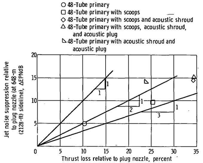
Figure 21. - Suppressor effectiveness. Flyover results scaled to four 267-kN-thrust engines; exhaust nozzle pressure ratio,  $P_8/p_0$ , 2.4; relative jet velocity,  $V_r$ , 533 m/sec (1750 ft/sec); corrected secondary rate flow ratio  $\omega\sqrt{T}$ , 0.06; Flight Mach number,  $M_0$ , 0.4.
