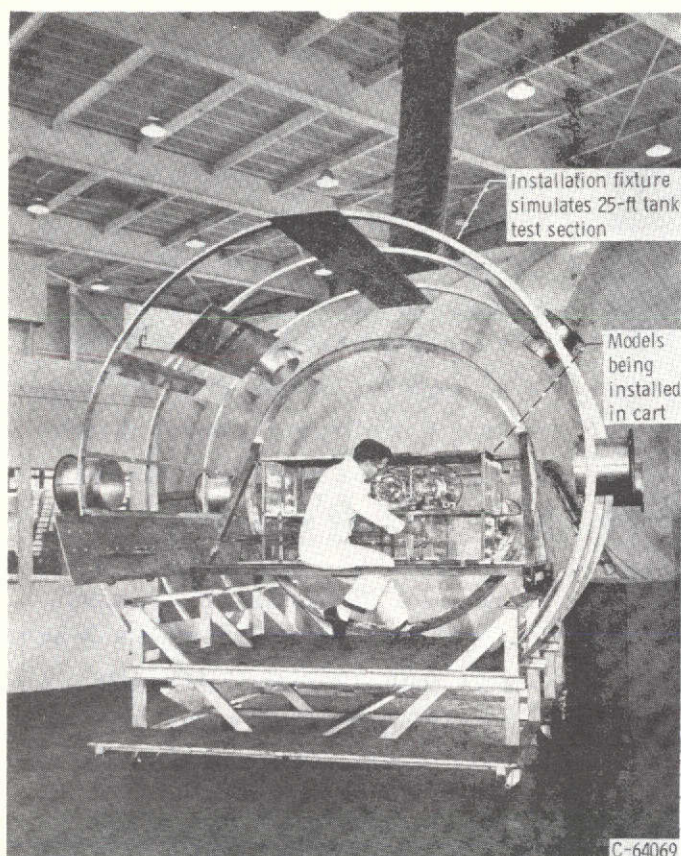
Figure 10. - Thrustor installation in cart and installation fixture.
