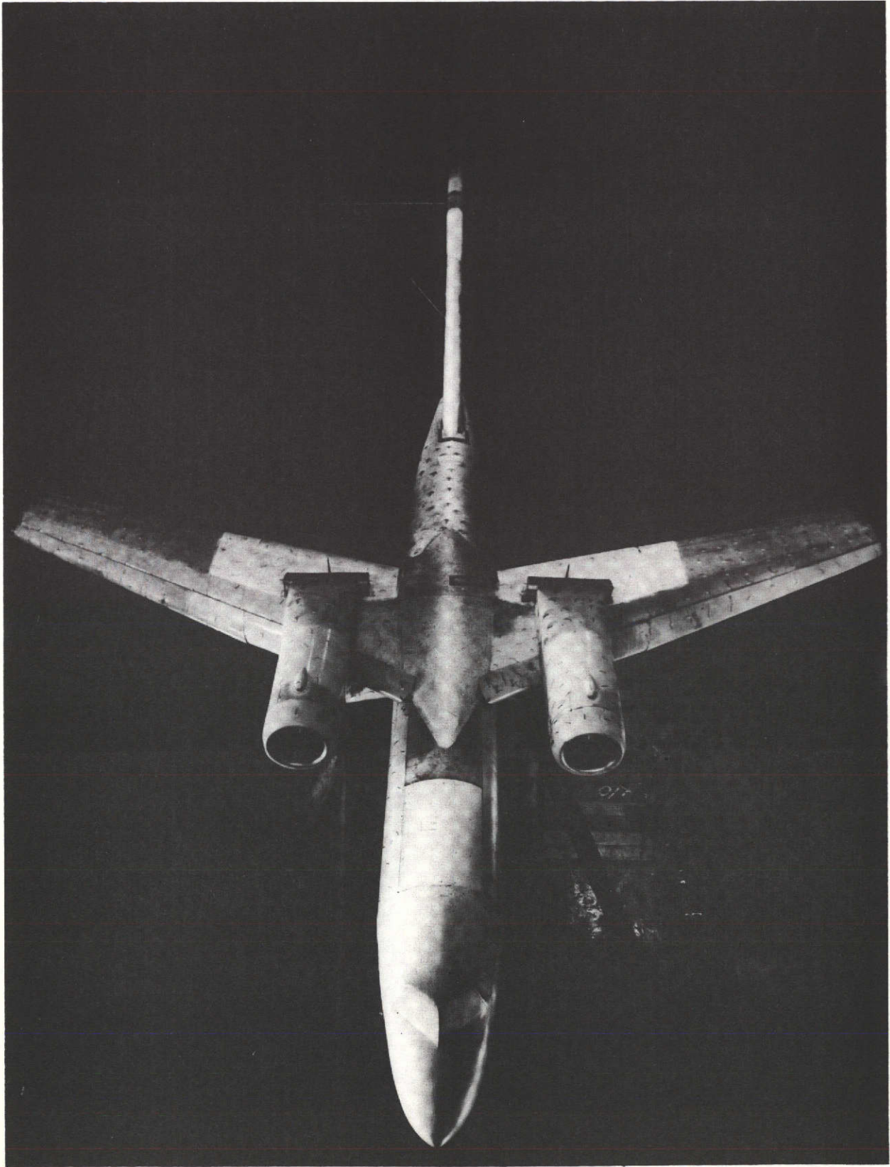
(a) Top view of model installed in wind tunnel.
