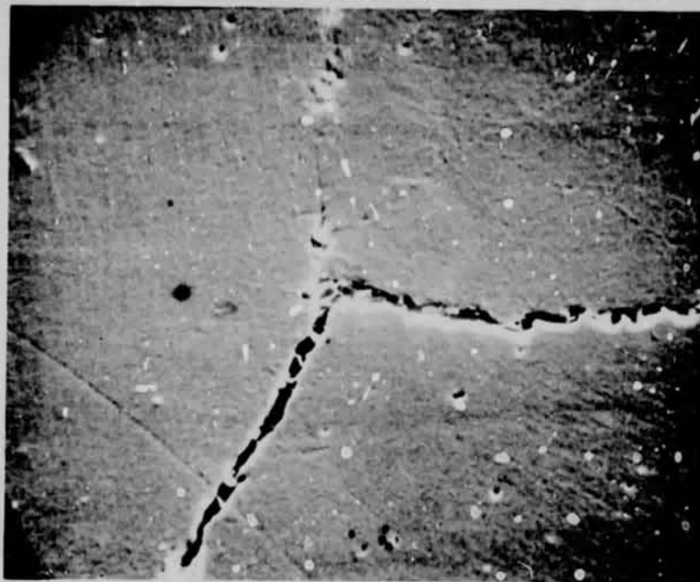
(a) Grain boundary decohesion in interior of specimen approximately 1.8mm below fracture surface. 2000X
