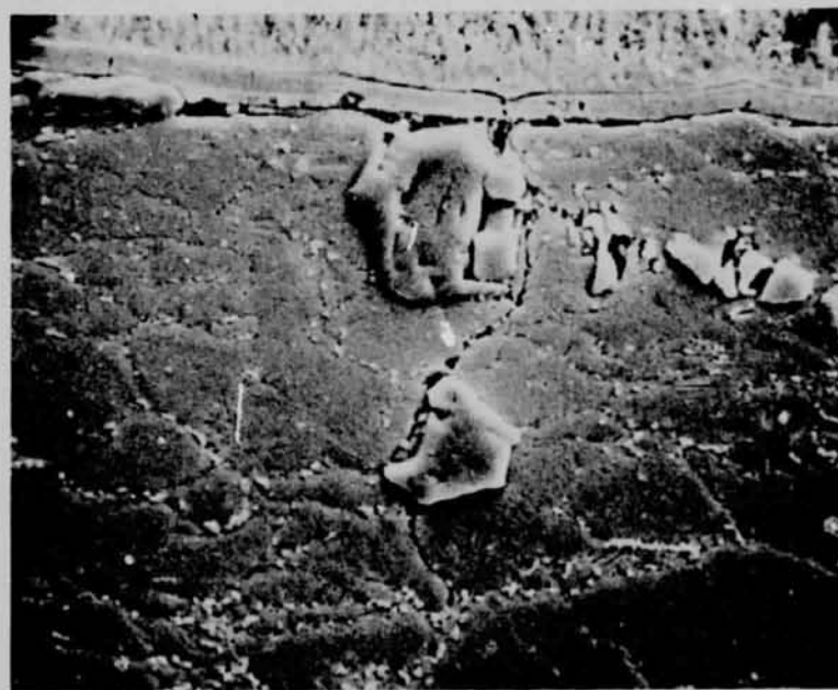
(b) Secondary crack approximately 1.8mm below fracture surface.
