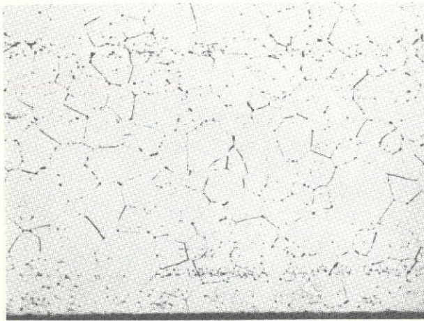
(a) Specimen T-T-1, taken from heater inlet, about 1175° C (2150° F).
