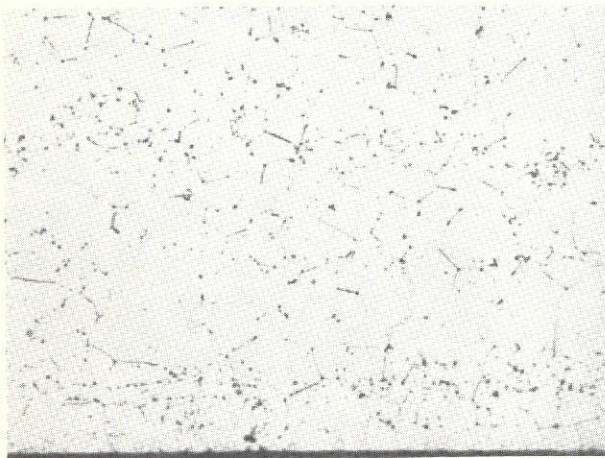
(a) Specimen T-C-16, taken from near heater inlet, about 1165° C (2130° F).
