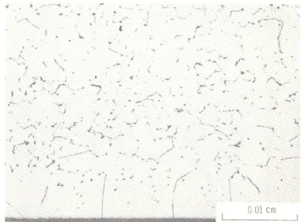
(b) Specimen A-T-5, taken from heater exit, about 1360° C (2475° F).
