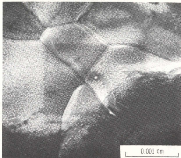
(c) Specimen A-C-2, exposed to lithium at about 1350° C (2460° F).
