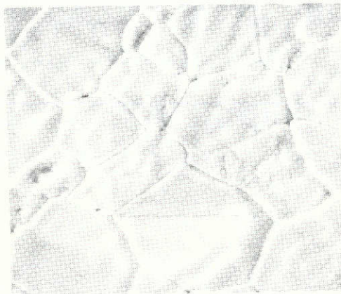
(a-2) Specimen T-T-10, exposed to lithium at about 1205° C (2200° F).
