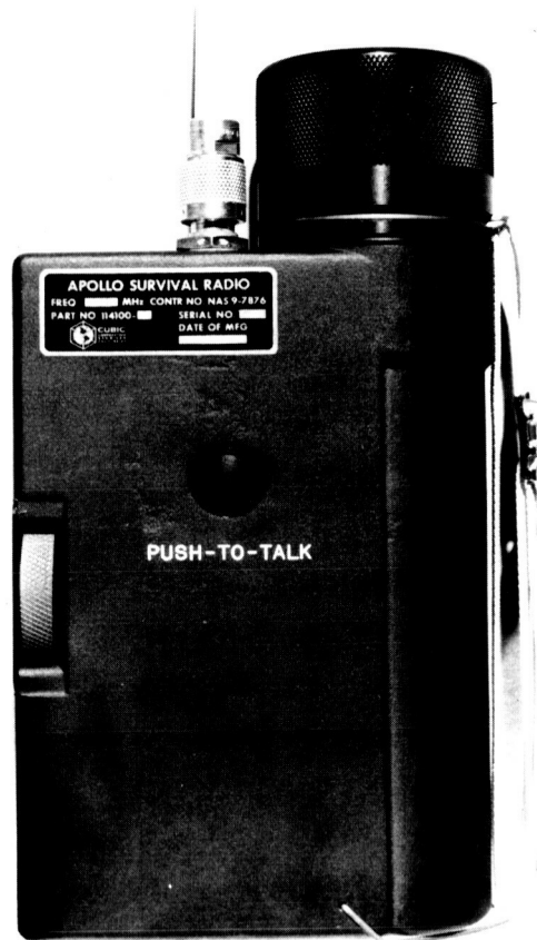
Figure 5.- Front view of Apollo survival radio.
