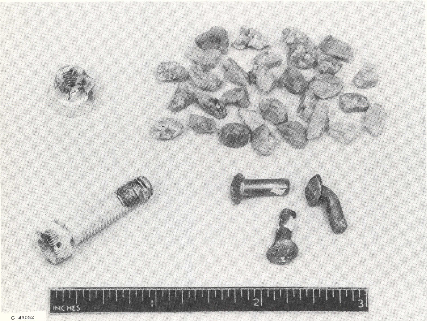
FIGURE 5. SMALL IMPACT MEDIA FOR FOD TESTING
