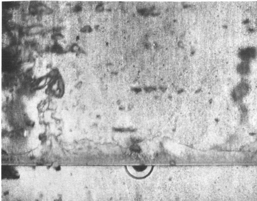
(b) 0.051-Centimeter-diameter heater; 70.4 centimeters per second. Figure 8. - Refrigerant 113 boiling at heat flux just below burnout.
