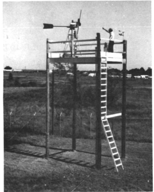
Figure 10. Photograph of the 500 watt experimental prototype wind energy storage system mounted on a twenty foot platform.
