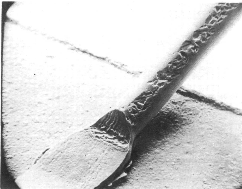
b: Wire has twisted after being clamped and before bonding so that the clamp marks are incorporated in the weld interfacial region.
