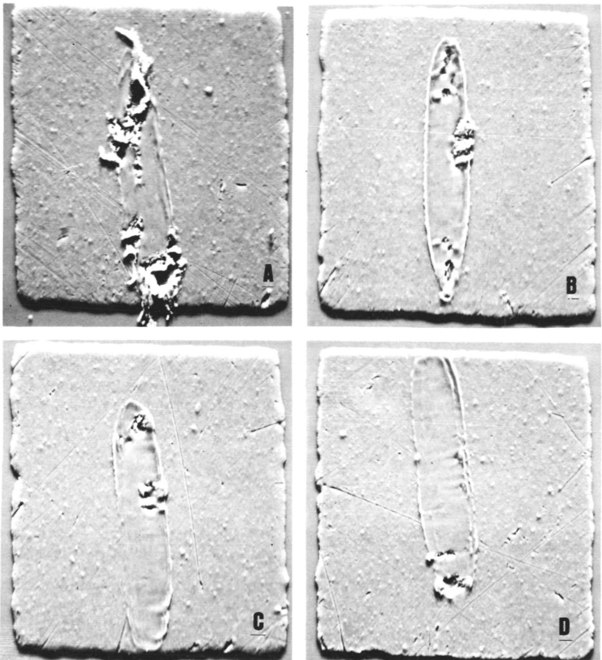
Fig. 3-12. SEM photomicrographs (460X) of bond lift-off patterns for first bonds made at different time settings and constant power setting. The time is longest for case (a) and is decreased to the shortest value for case (d). Settings used in case (a) result in a bond which will adhere to the pad; the shorter time settings do not produce an adherent bond. The scratches on the bonding pads (which result from a cleaning process no longer in use) are smoothed out by the impact of the tool compressing the wire against the pads before ultrasonic energy is applied. Note also the apparent movement during bonding exhibited in case (d). This results from mechanical vibration in the bonding machine.
