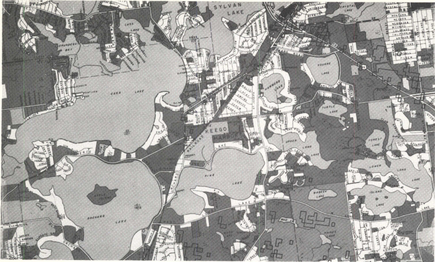
Fig. 9 ERTS computer-generated overlay of extractive earth boundaries on Oakland County land-use map (scale 1:48, 000).
