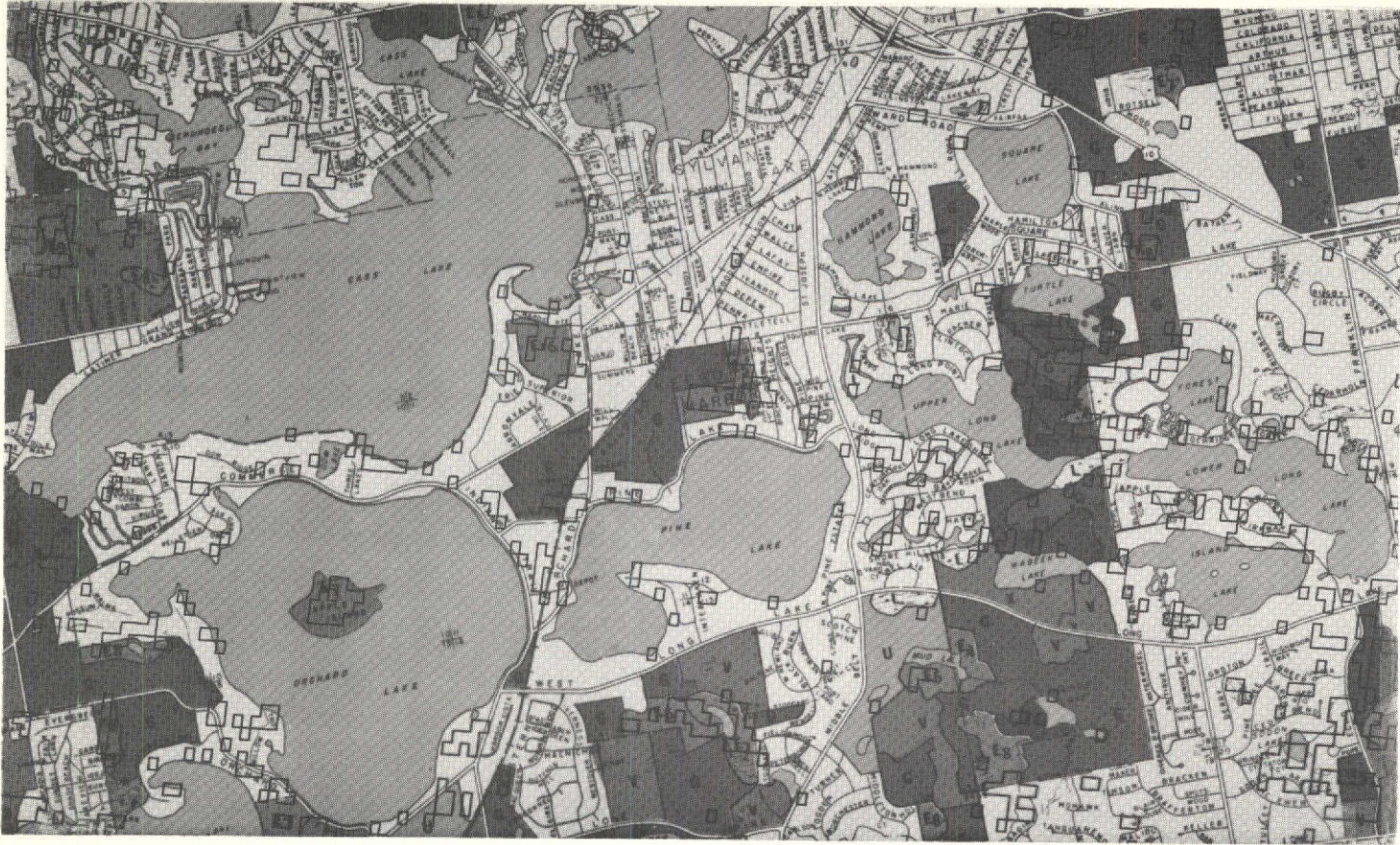
Fig. 7 ERTS computer-generated overlay of forested land boundaries on Oakland County vegetation map (scale 1:48,000). Map symbols E, K, M denote deciduous forest.
