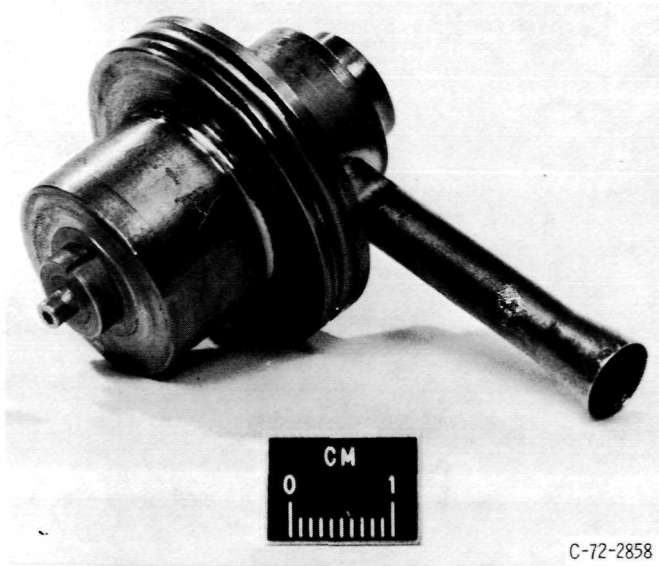
(c) Bare assembled diminiode.
