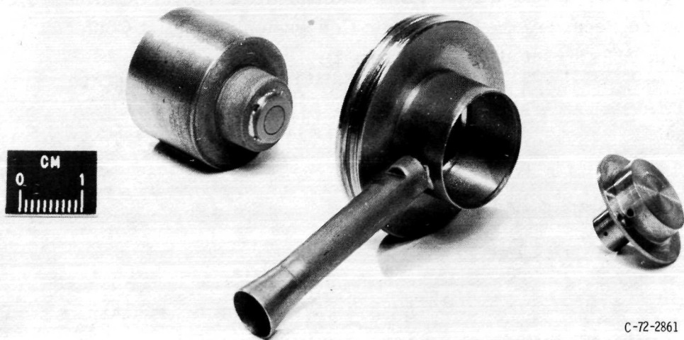
(b) Collector, envelope, and emitter sections of diminiode.
