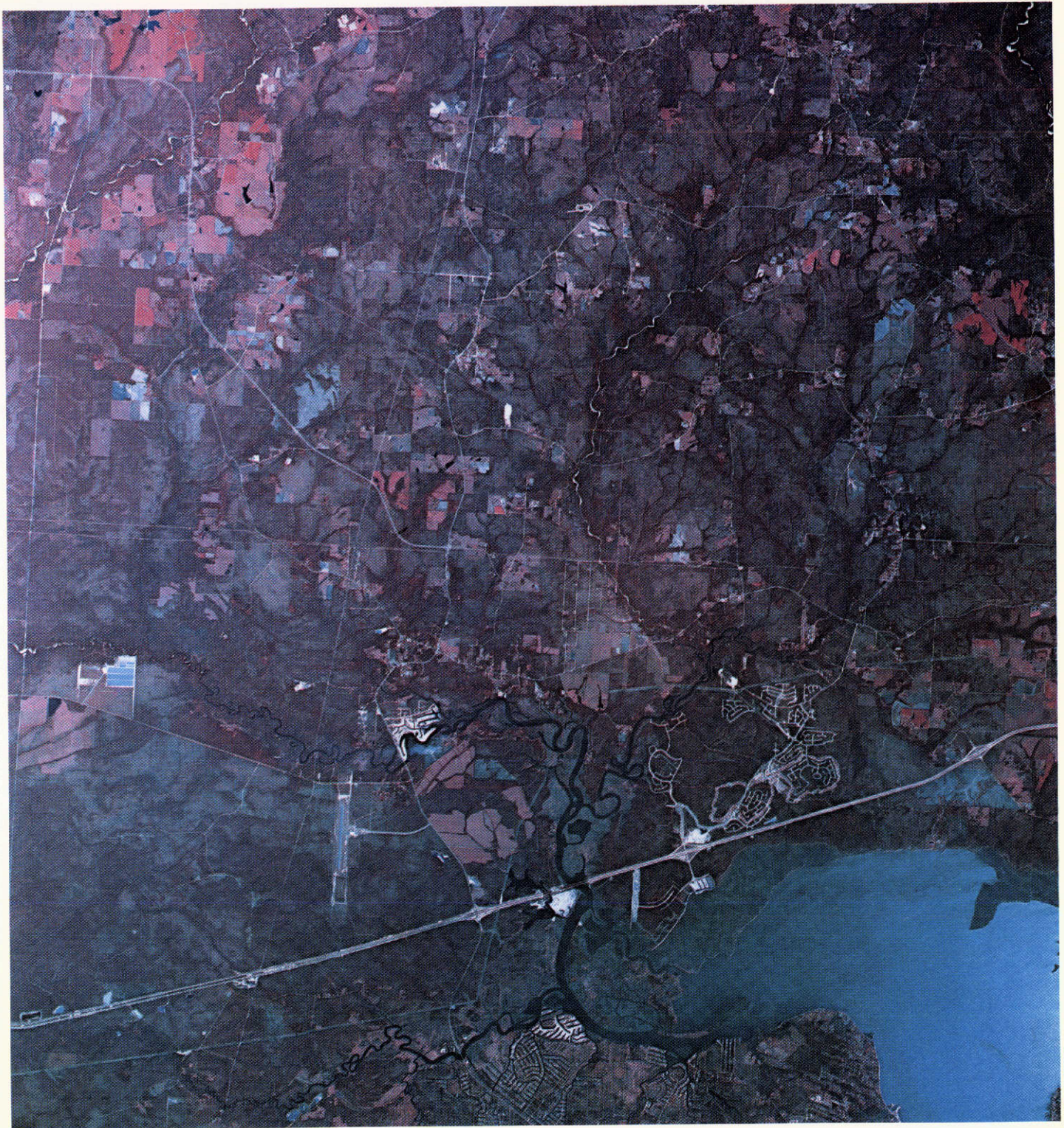
Figure 1.- Aerial, color infrared photograph of a portion of Hancock County, Mississippi, taken from an altitude of 18 300 meters (60 000 feet) with a 15.24-centimeter (6 inch) focal-length camera (scale of original, 1:120,000).
