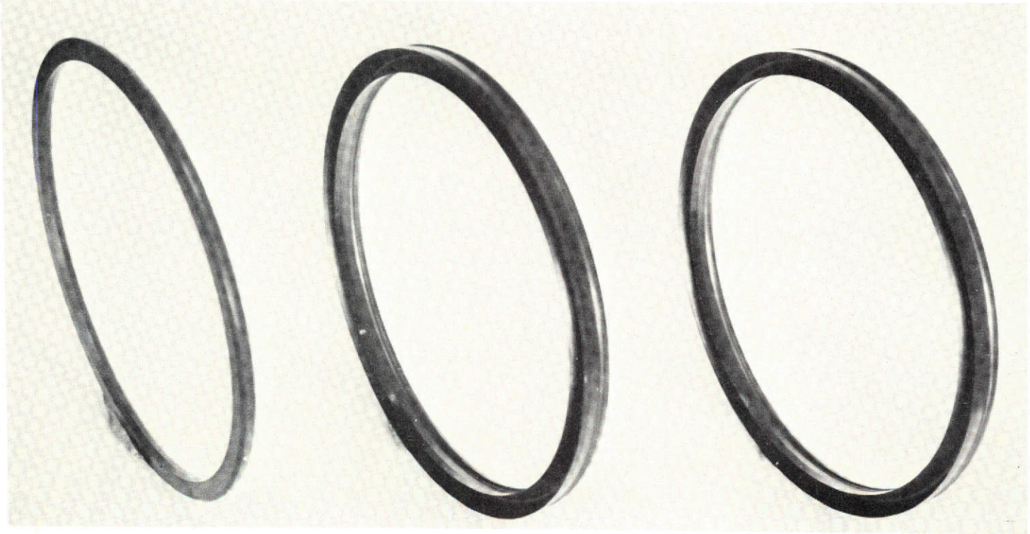
FIGURE 12.—K-SECTION SEAL AT TEST COMPLETION
