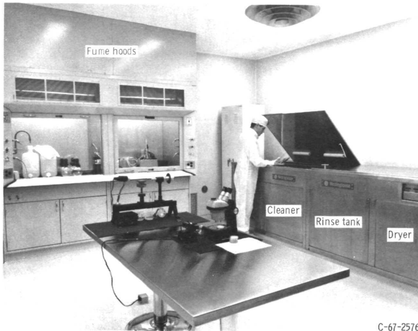
(a) Ultrasonic cleaning system.
