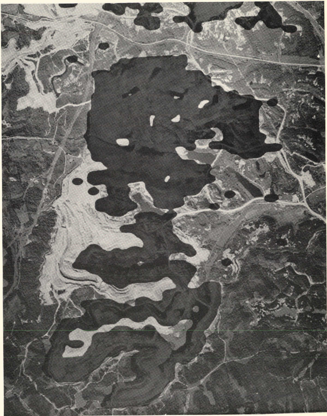
Figure 9 Stripped Earth Category (Red) Generated from 21 August 1972 ERTS Tape Overlaying Aerial Photograph Acquired on 7 September 1973
