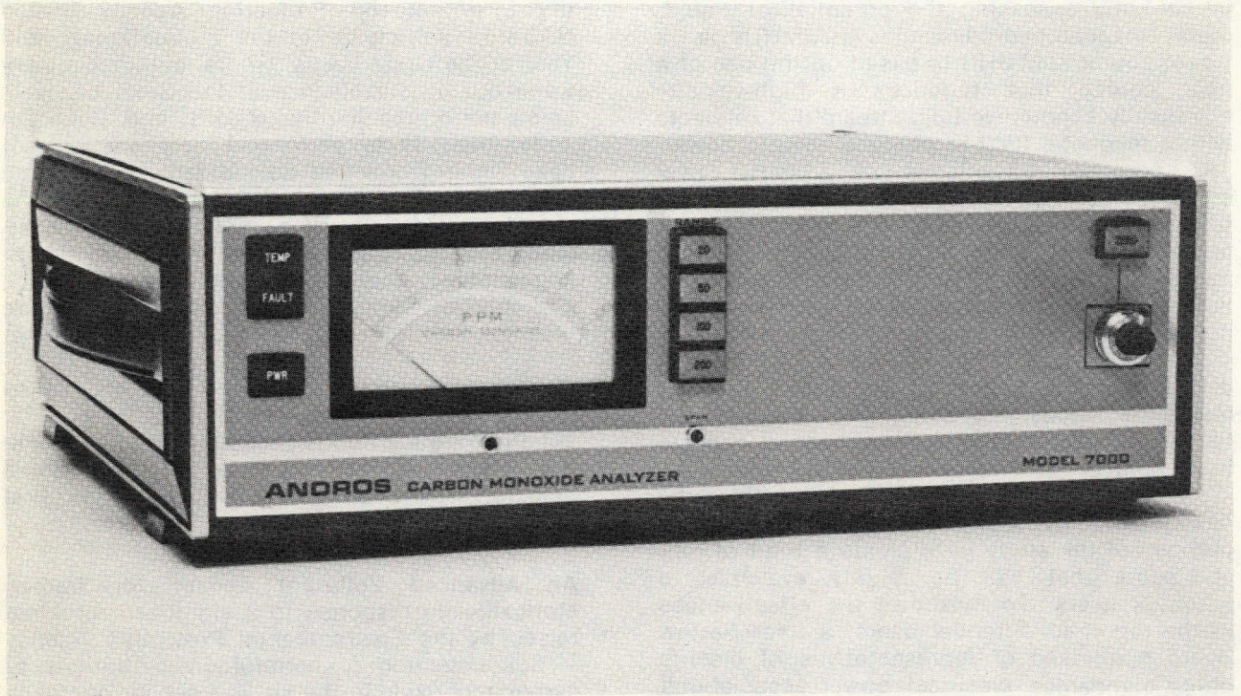
Figure 3. Now commercially available from Andros Incorporated of California, this device detects and measures carbon monoxide in the air. It was adapted from hardware originally designed for use in the NASA Skylab program to monitor space-cabin carbon-monoxide concentrations.
