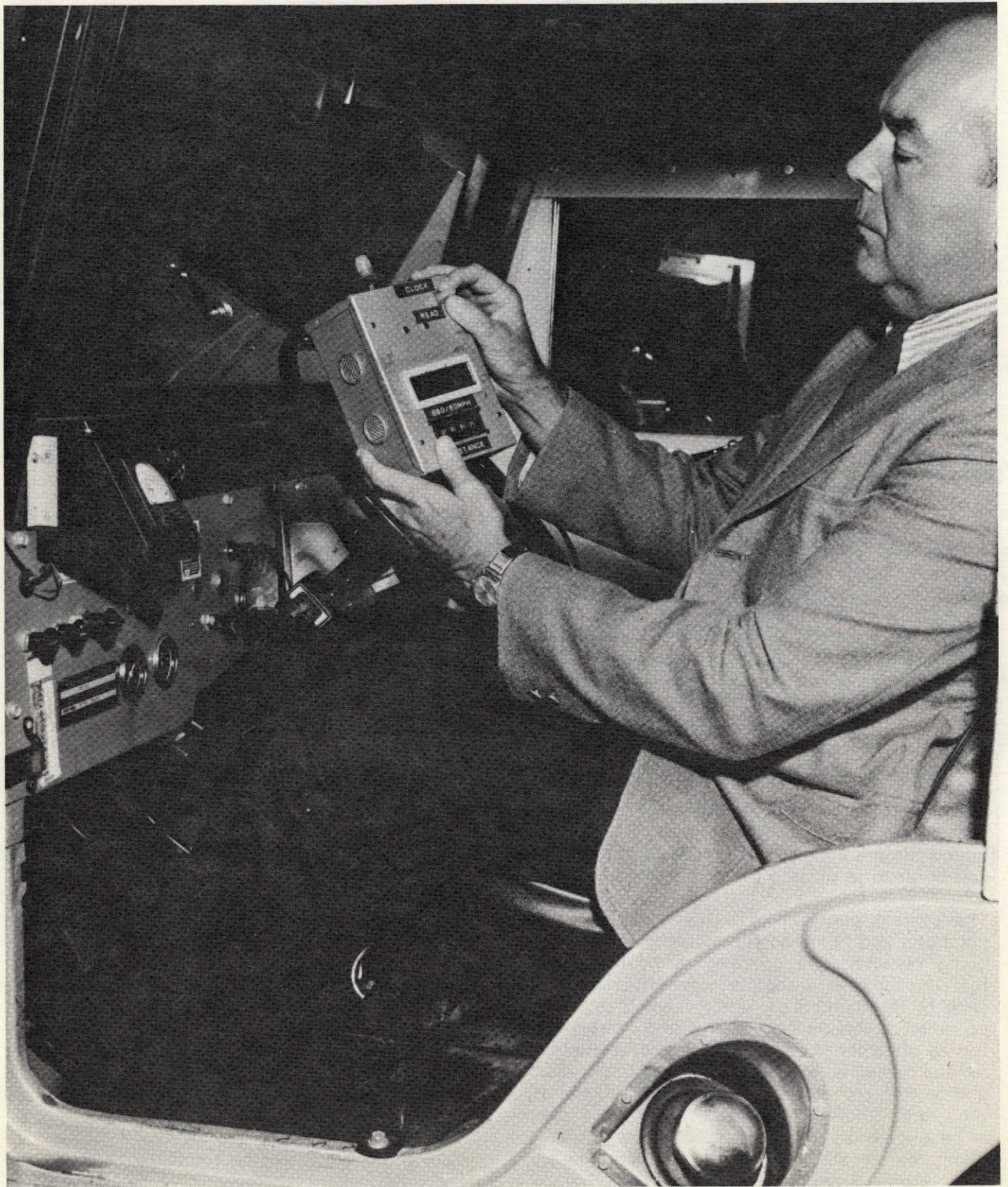
Figure 12. Low-cost, simple, minicomputerized road-speed monitoring system based on aerospace technology is being used in Huntsville, Alabama, home of the inventor, an engineer at Marshall Space Flight Center. System can be installed in police cars or at roadside.
