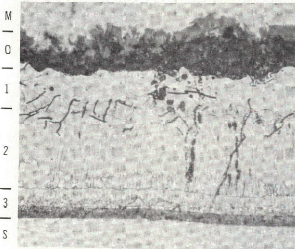
(a) R512E coated Cb-752 after 5 cycles.
