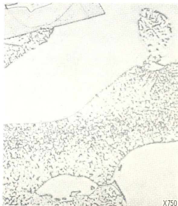
(b) Aged 100 hr at 982°C (1800°F) plus 500 hr at 871°C (1600°F).
