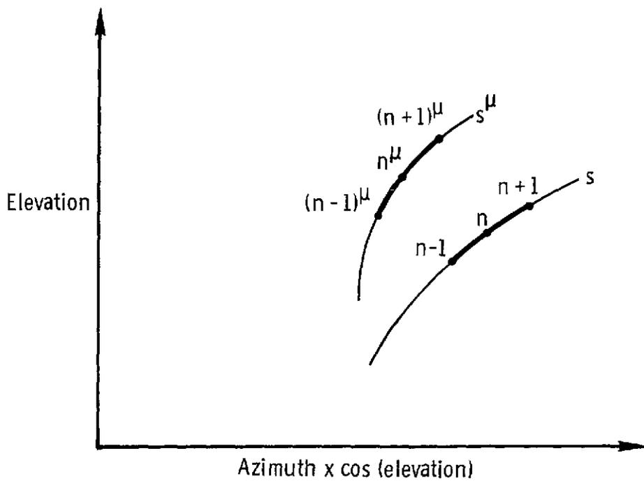
Figure 1.- From observation station  $\mu$ , image trace segment  $(n-1)^\mu$ ,  $n^\mu$ ,  $(n+1)^\mu$  differing from error-free trace segment  $n-1$ ,  $n$ ,  $n+1$  in location, orientation, and shape.
