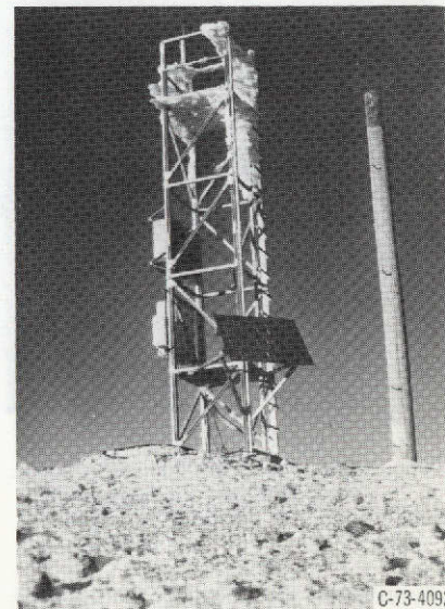
Fig. 6 - Solar cell powered RAMOS weather station on Mammoth Mountain, CA.
