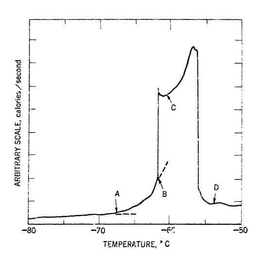
FIGURE 2. - Thermogram for a Frozen A-50/NTO Mixture for a Heating Rate of 5° F/min.
