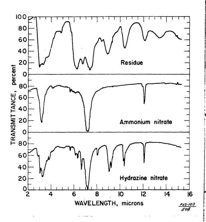
FIGURE 3. - Infrared Spectra of Residue from  $N_2H_4/NTO$  Reaction, Ammonium Nitrate, and Hydrazine Nitrate.
