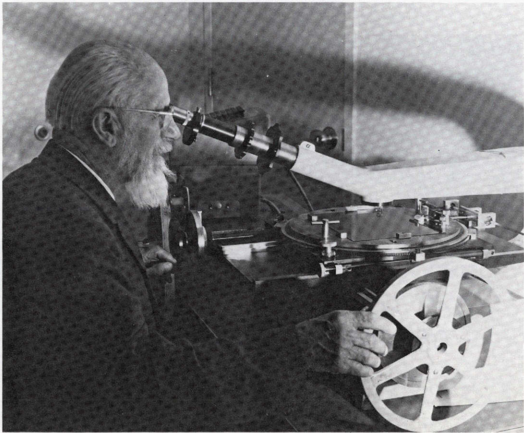
Figure 2: Dr. George Van Biesbroeck of the Lunar and Planetary Laboratory, University of Arizona, finding the accurate position of an image on a photographic plate, using a Mann Measuring Engine. (Courtesy R. B. Minton, Lunar and Planetary Laboratory, University of Arizona.)
