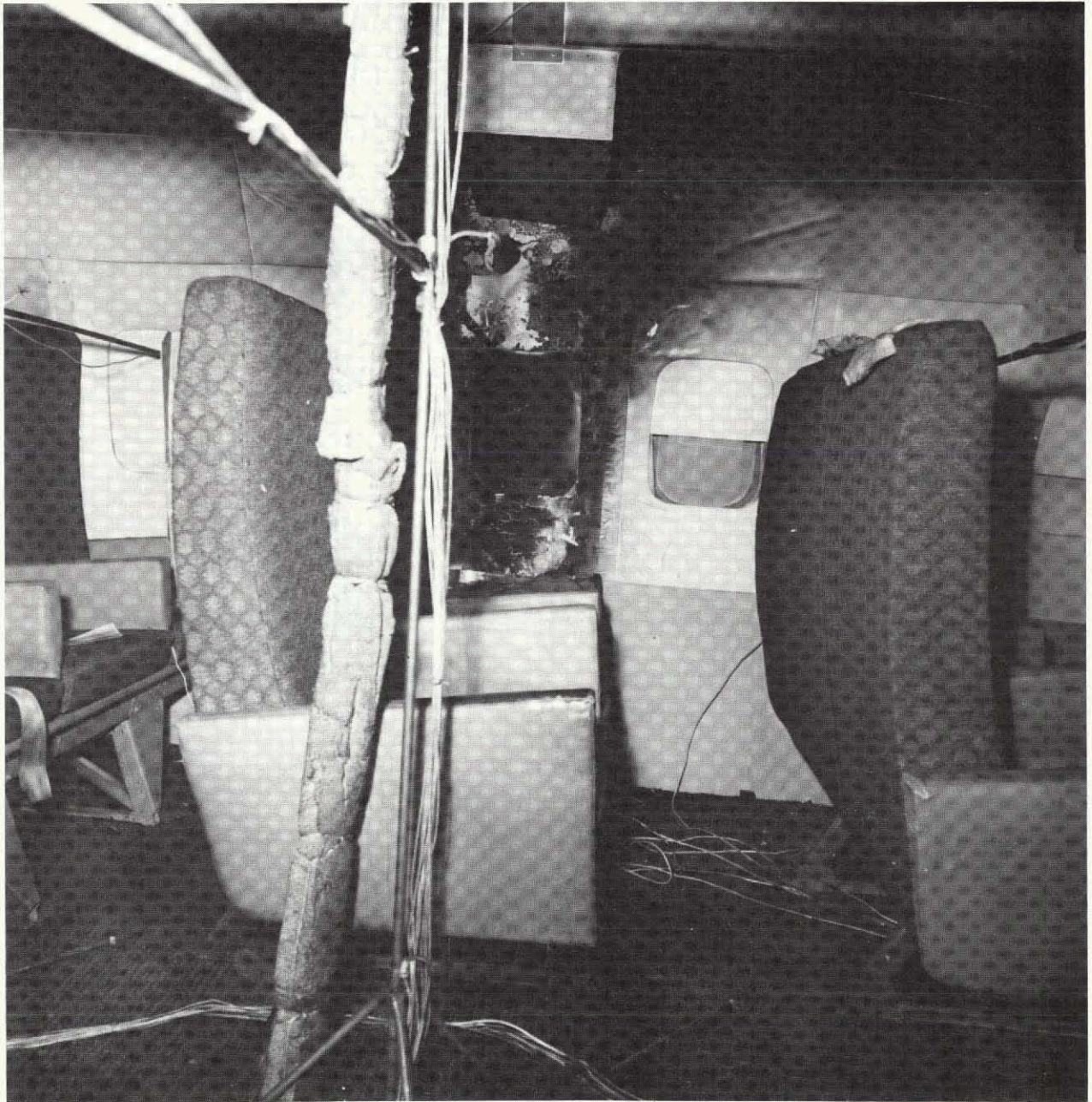
Figure 20.- Fire damage for test 2 using new materials, side view.
