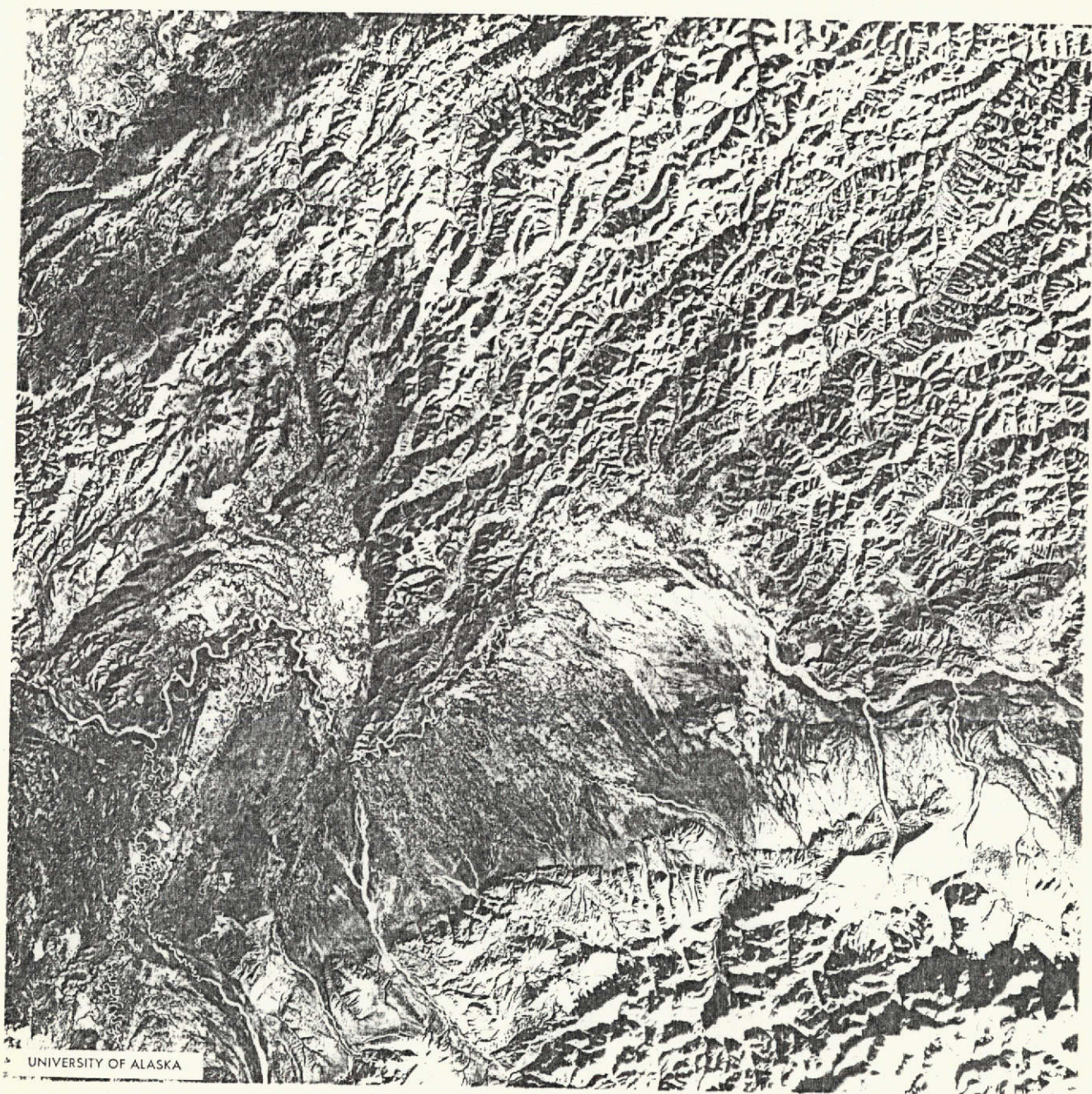
Figure 14. Mosaic of 6 ERTS images sidelapping previous mosaic to the east. For stereoscopic viewing with Fig. 13, there is a narrow strip down the (composite) scene for which both mosaics employ the same pass, and the sensation of relief would not be expected. However, even outside this area, the stereoscopic effect is minimal.
