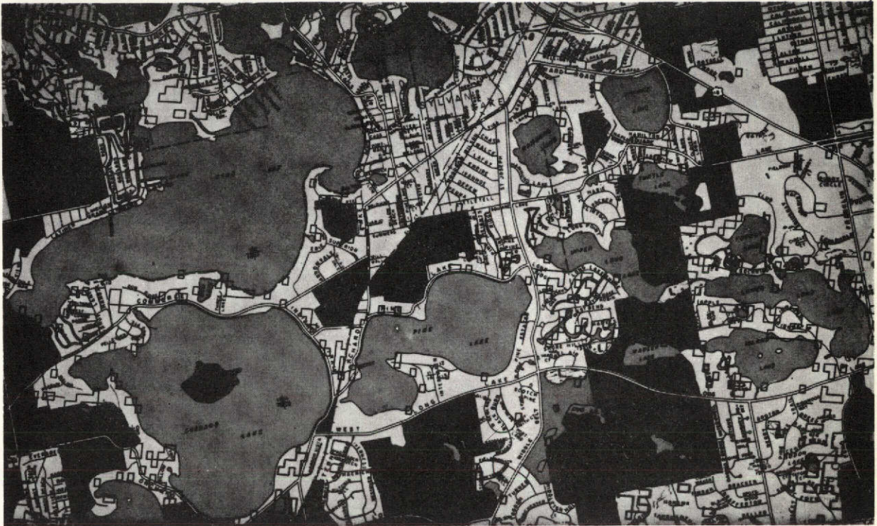
FIGURE 5. ERTS COMPUTER-GENERATED OVERLAY OF FORESTED LAND BOUNDARIES ON OAKLAND COUNTY VEGETATION MAP (SCALE 1:48,000). Map symbols E, K, M denote deciduous forest.
