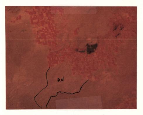
Fig. 16. Color print from photograph of ERTS composited bands 5 and 7 in St. Anthony dunes area. Unit 2d shows elongated dunes as light colored lineations with sparse vegetation and interspaced with grey areas supporting normal vegetation on clay soils.
