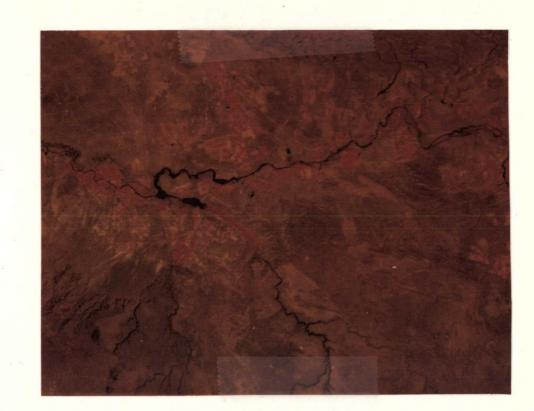
Fig. 14. October 1972 ERTS imagery shows a portion of the Mountain Home-Jarbidge area. At this date there is less color because of decreased photosynthetic activity and the topographic relief features are much more pronounced.
