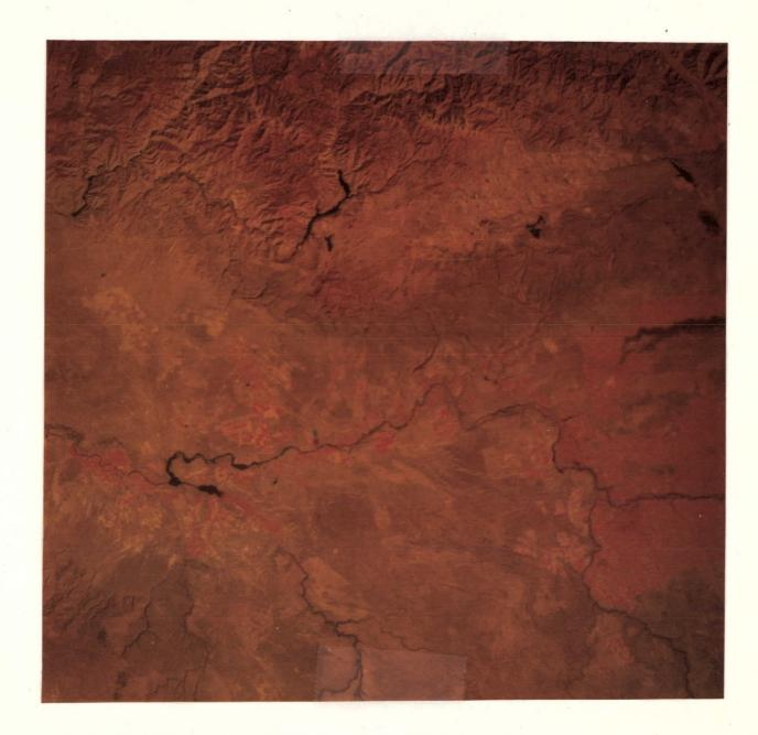
Fig. 5. Color enhanced ERTS-1 imagery from bands 5 and 7 using green and red filters, respectively. This combination yielded highly interpretable imagery of vegetation, water bodies, landform, geology and soils.
