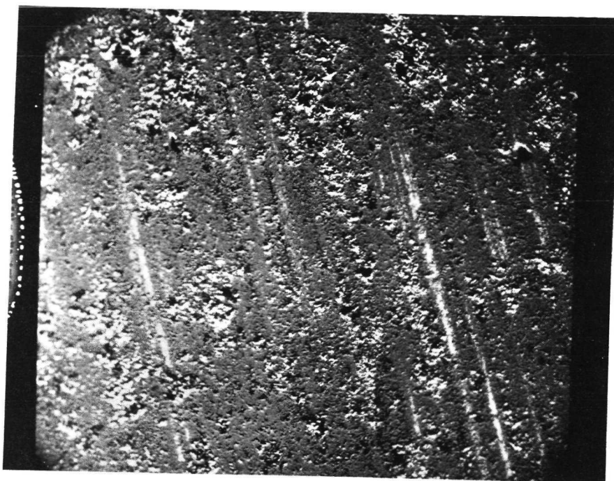
Pad After Testing - 100X Electron Back Scatter Composition
