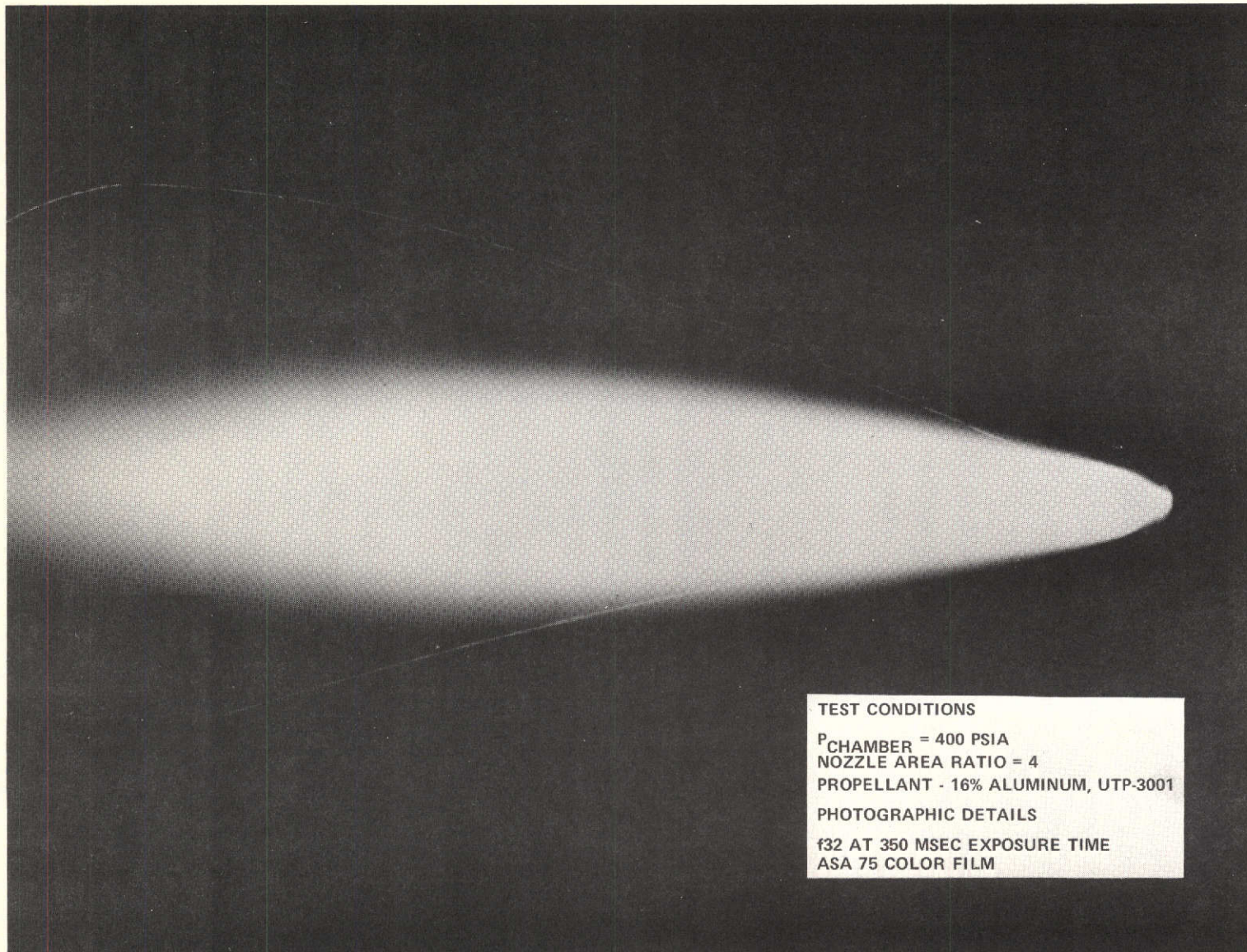
Figure 15 TIME EXPOSURE PHOTOGRAPH OF A SOLID PROPELLANT ROCKET PLUME
