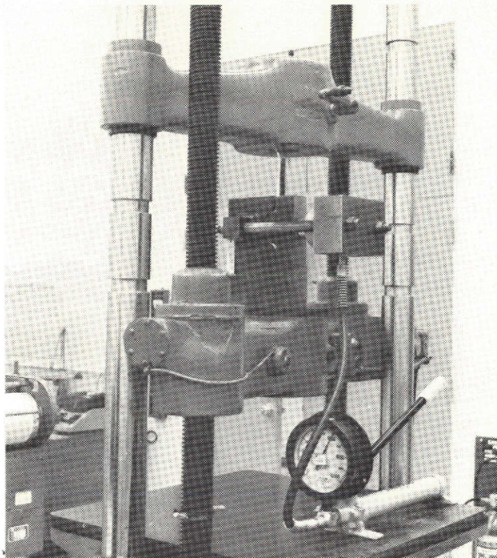
Figure 3-2. View Showing Test Fixture in Tensile Tester
