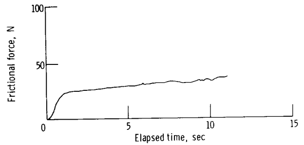
Figure 7. - Constant-speed friction trace for hot isostatically compressed nickel - 30-percent gadolinium oxide composite. Normal load, 220 newtons (82 N/cm 2 ); sliding speed, 100 feet per second (31 m/sec).
