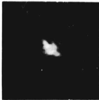
FIGURE 10. MAGNIFIED VIEW OF POINT FOCUS PRODUCED BY THE FIRST HOLOGRAPHIC OPTICAL ELEMENT AT f/20
