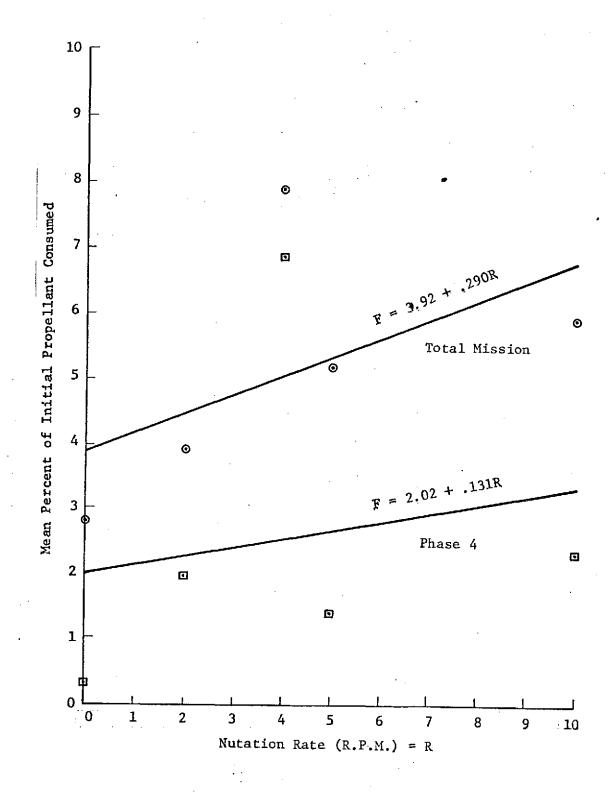
FIGURE 5. Mean Percent of Initial Propellant Consumed as a Function of Nutation Rate
