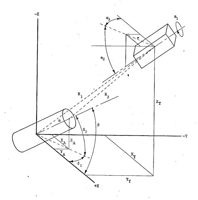
FIGURE 7. Satellite-Teleoperator Geometry
