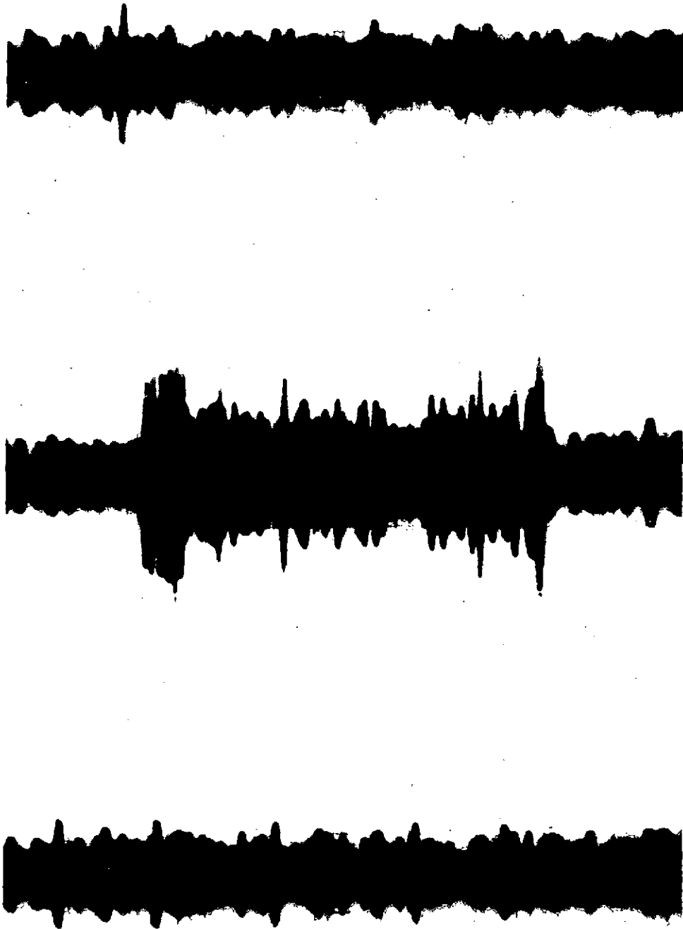
Figure 1 -- Oscilloscope photographs of a Jovian S-burst (center trace) and an isolated micropulse (top trace). These photographs represent 100 kHz-bandwidth IF output of an 18 MHz receiver as recorded in 1967.
