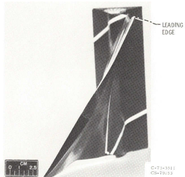
Figure 2. 2200 FT/SEC TIP-SPEED COMPRESSOR BLADE SHOWING NONLINEAR TWIST
